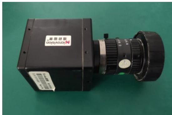
**Figure 1.** Camera for image acquisition.
