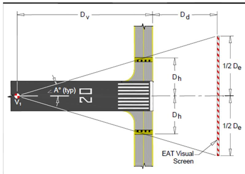
Figure 15. End-around taxiway screen sizing and location [67].
