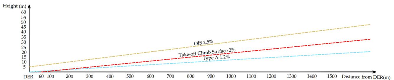
Figure 13. The comparison of OIS, take-off climb surface, and type A surface in the vertical direction.
