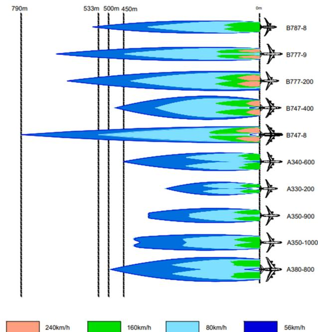
**Figure 12.** Typical aircraft jet blast impact range of taking off [17].
