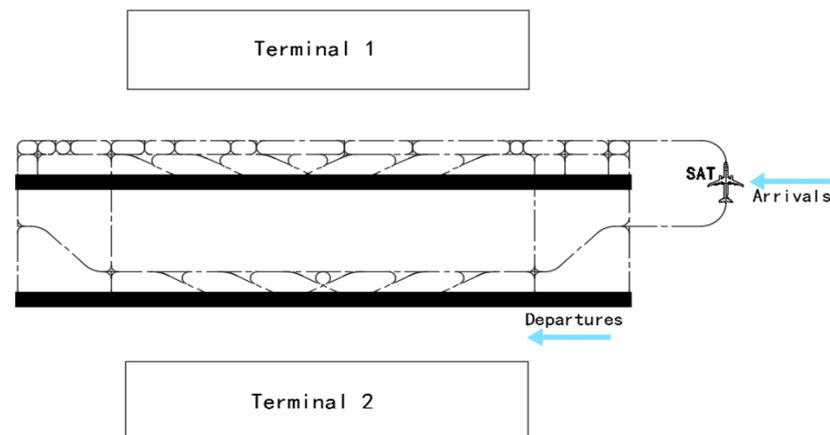
**Figure 10.** Example of typical SAT operation.
