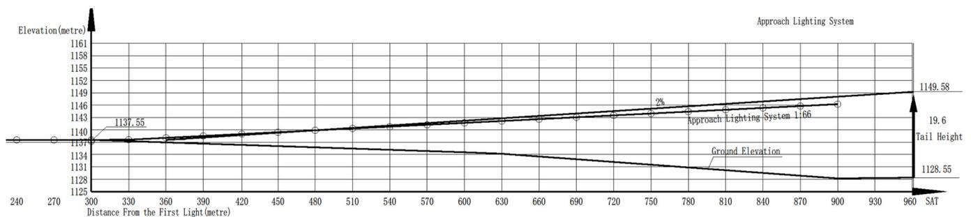
Figure 16. The elevation of approach lighting system and sunken end-around taxiway of KWE.
