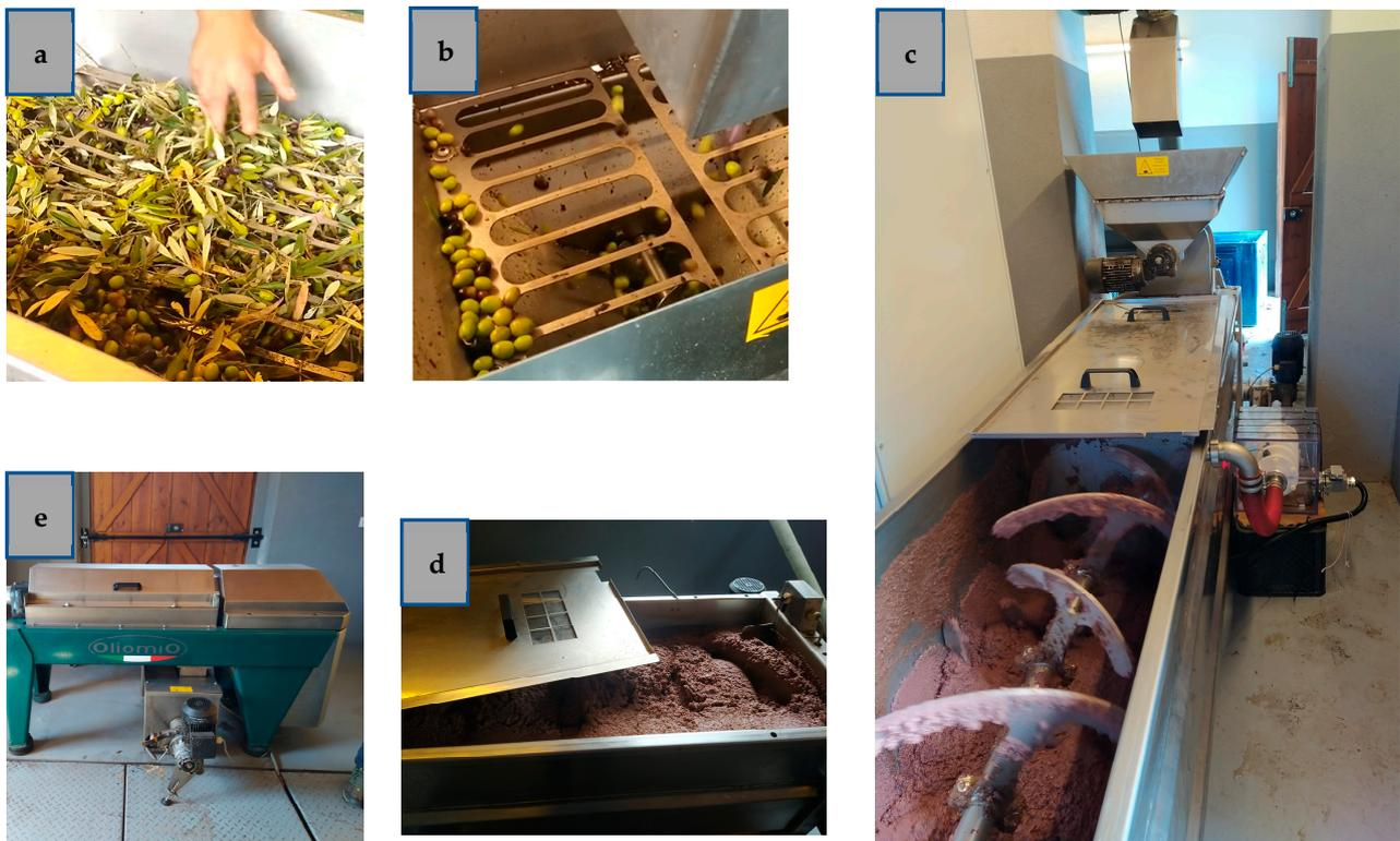
**Figure 1.** Steps of olive oil extraction line with the PEF chamber before the malaxer container. (a) Cleaning; (b) crushing; (c) PEF treatment; (d) malaxation; and (e) centrifugation.
