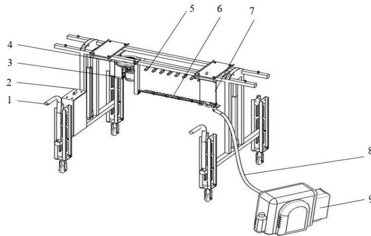
**Figure 1.** Overall structure diagram of tea harvester: (1) handle; (2) control box; (3) motor; (4) fan; (5) leaf-collecting pipeline; (6) cutter; (7) telescopic devices; (8) soft shaft; (9) gasoline engine.
