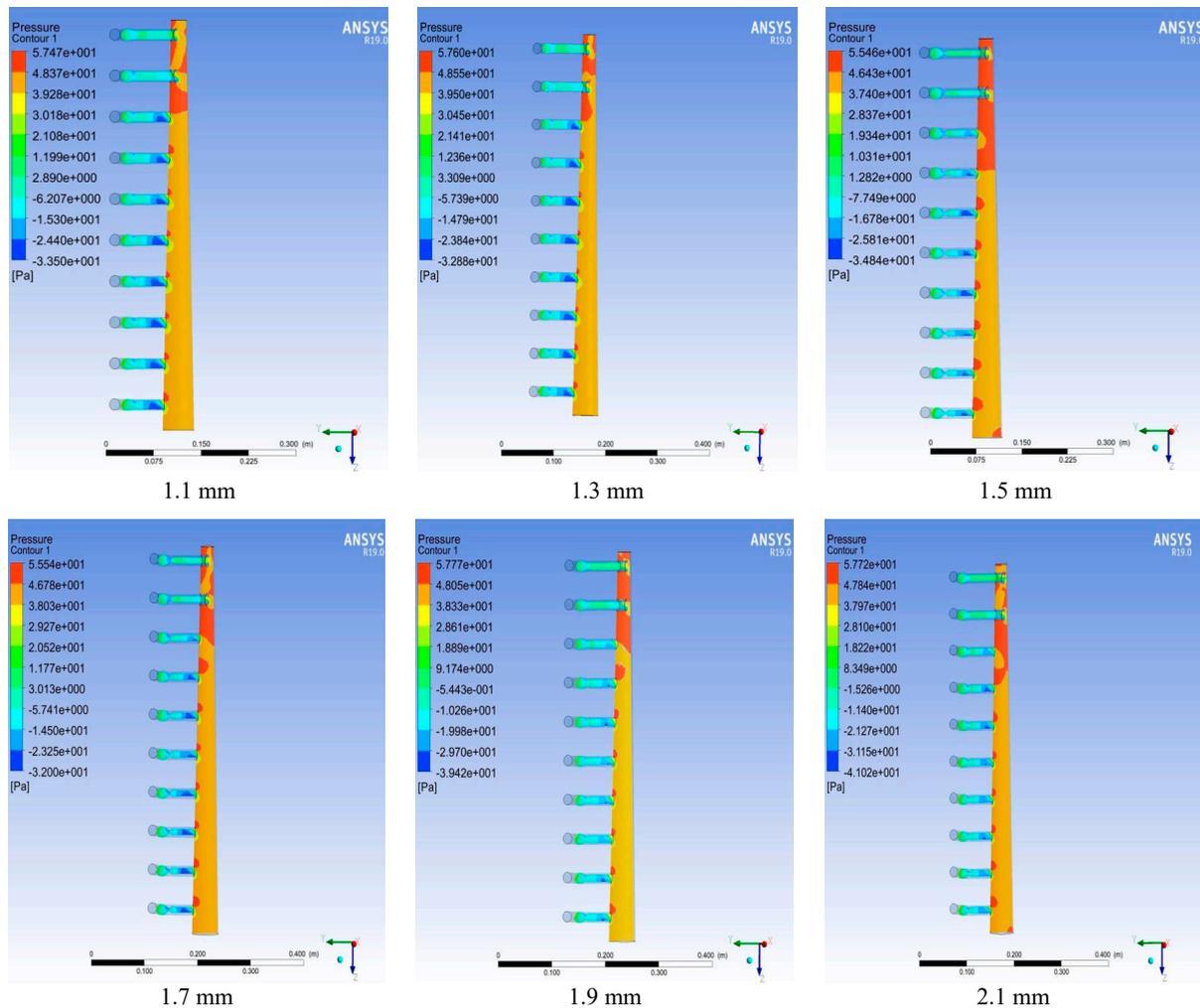
**Figure 11.** Pressure cloud map with different extension lengths.
