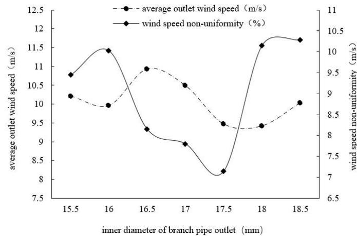
**Figure 6.** Effect of inner diameter of branch outlet on average outlet wind speed and wind speed non-uniformity.
