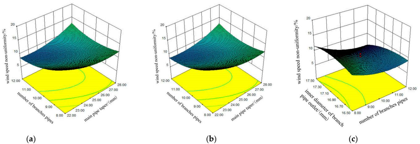
**Figure 8.** Response surface of various factors on the non-uniformity of wind speed: (a) C = 17 mm; (b) B = 10; (c) A = 25 mm.
