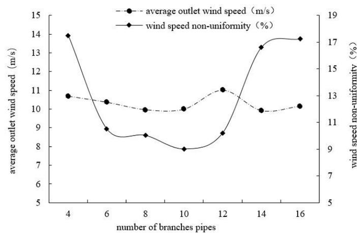
**Figure 5.** Effect of number of branch pipes on the average outlet wind speed and wind speed non-uniformity.
