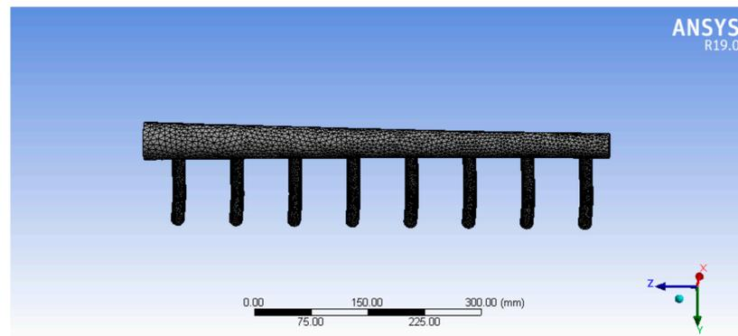
**Figure 3.** Mesh division of the leaf-collecting pipeline.
