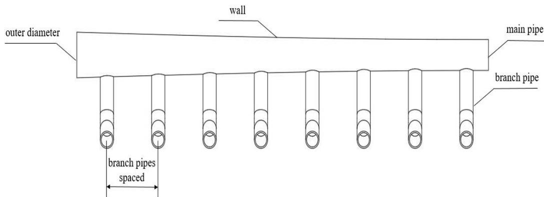
**Figure 2.** Three-dimensional view of the leaf-collecting pipeline.
