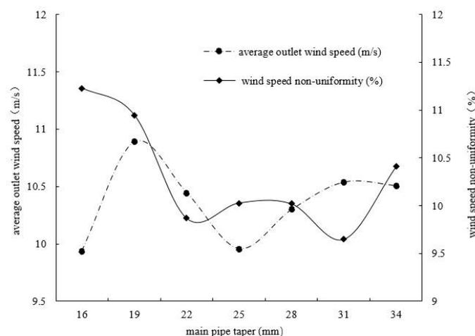
**Figure 4.** Effect of main pipe taper on average outlet wind speed and wind speed non-uniformity.
