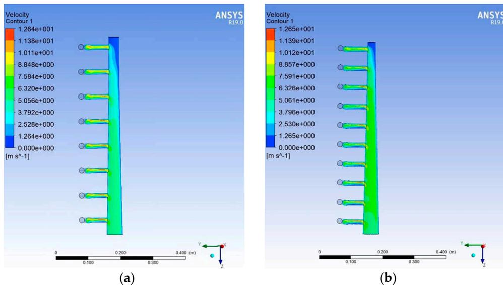
**Figure 9.** Speed cloud map of the leaf-collecting pipeline structure: (a) before optimization; (b) after optimization.
