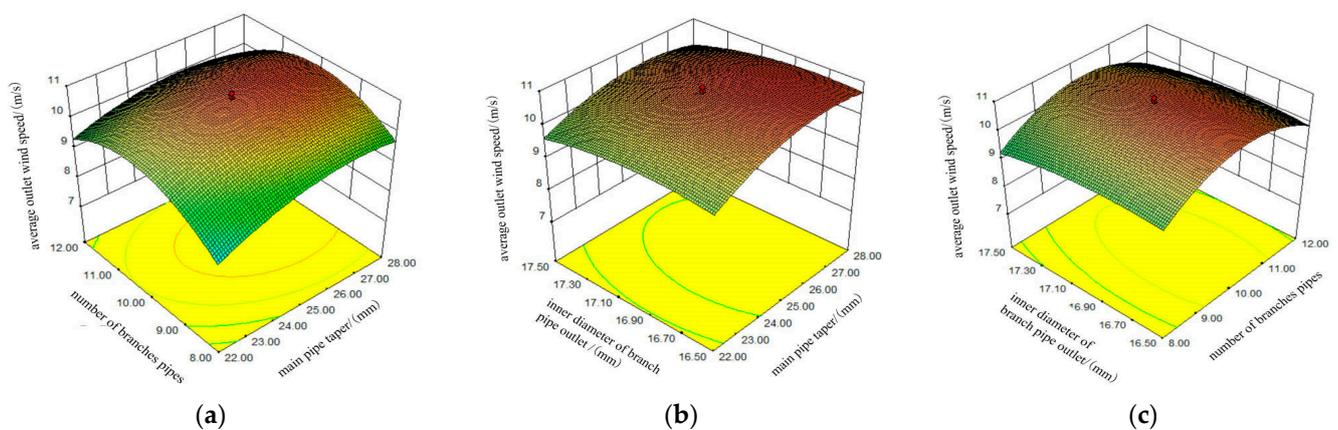
**Figure 7.** Response surface of the influence of various factors on the average outlet wind speed: (a) C = 17 mm; (b) B = 10; (c) A = 25 mm.
