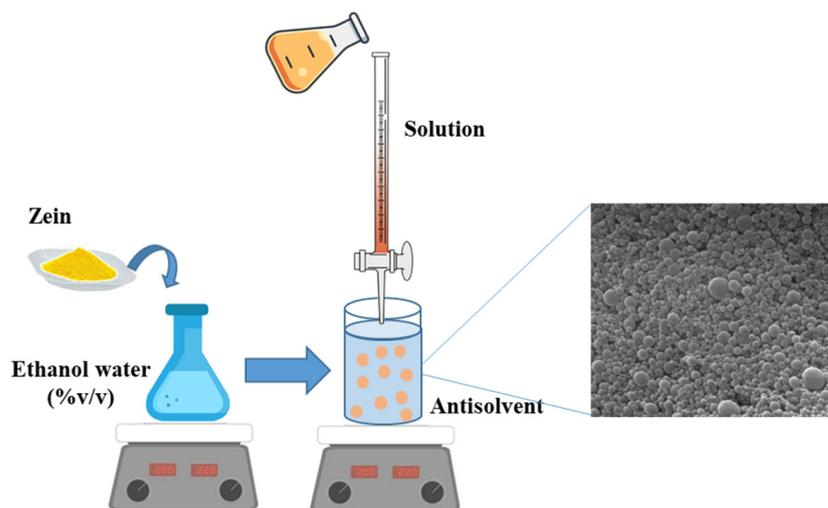
**Figure 3.** Schematic representation of the liquid antisolvent process and SEM image of zein NPs.
