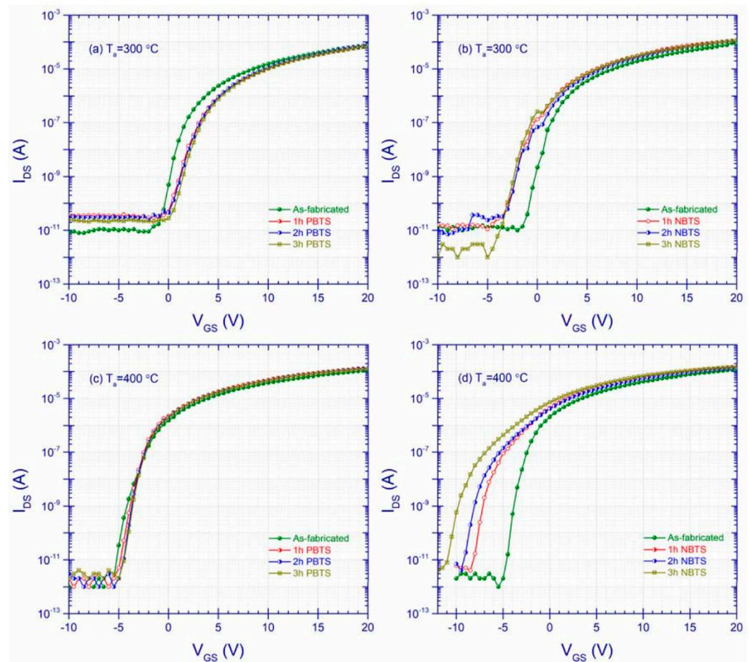
**Figure 6.** Transfer characteristic curves of the TFTs with IGZO annealed at 300 °C and 400 °C during 3h positive bias temperature stress (PBTS) and negative bias temperature stress (NBTS) (a–d).
