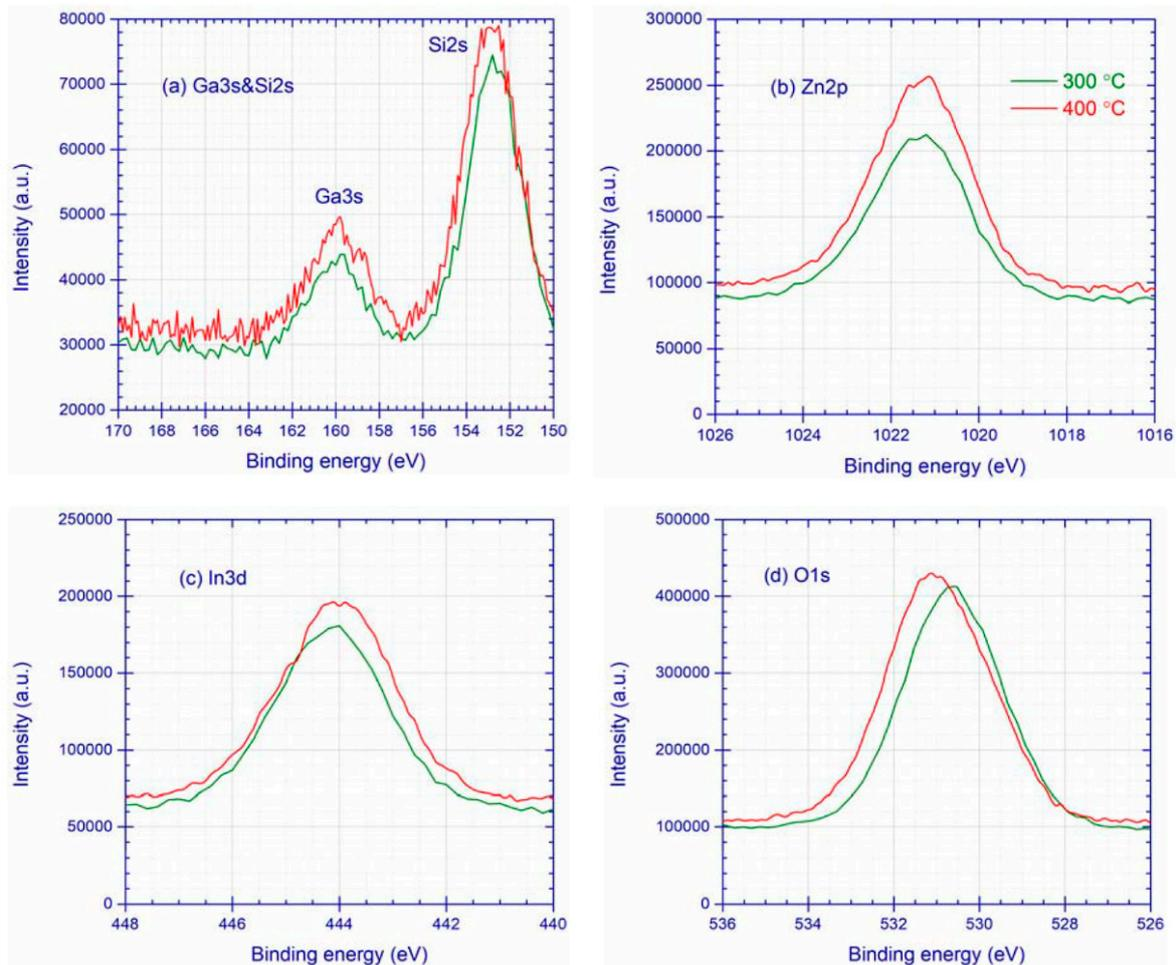
**Figure 3.** (a) Ga3s and Si2s, (b) Zn2p, (c) In3d, and (d) O1s spectra taken from IGZO-SiO<sub>2</sub> interfacial mixing layer annealed at 300 °C and 400 °C.
