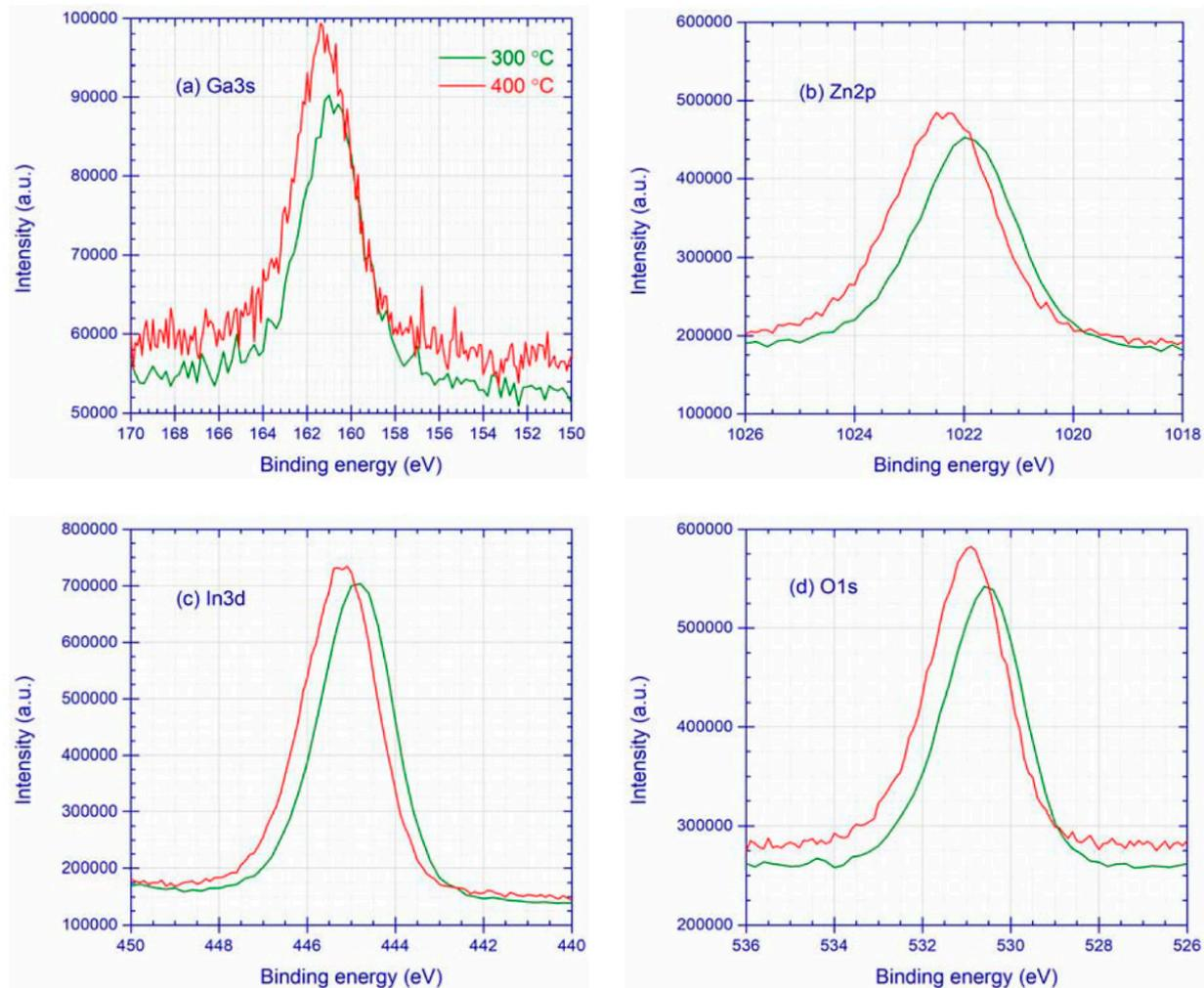
**Figure 2.** (a) Ga3s, (b) Zn2p, (c) In3d, and (d) O1s spectra of the IGZO layer annealed at 300 °C and 400 °C. The spectra were collected at a depth of 5 nm from IGZO surface.
