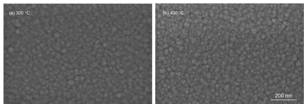
**Figure 5.** Surface morphology of IGZO annealed at (a) 300 °C and (b) 400 °C.
