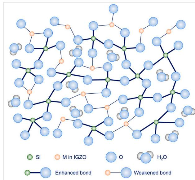
**Figure 7.** Schematic drawing of dual effects of higher  $T_a$  on structure of IGZO-SiO<sub>2</sub> mixing layer: enhanced Si-O bonds, weaker M-O bonds, and more H<sub>2</sub>O molecules.
