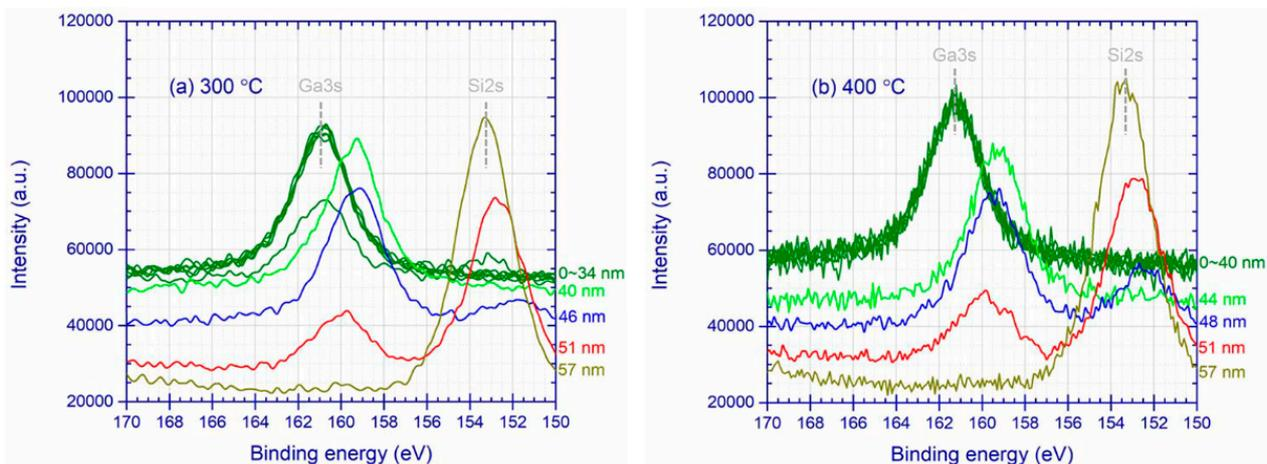
**Figure 1.** In-depth photoelectron spectra in the range of 150–170 eV for IGZO/SiO<sub>2</sub> samples annealed at 300 °C (a) and 400 °C (b).
