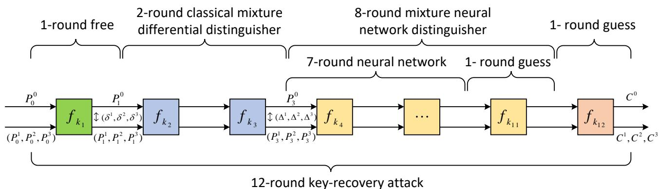
**Figure 6.** The 12-round key recovery attack using MDNN for SIMON32/64.
