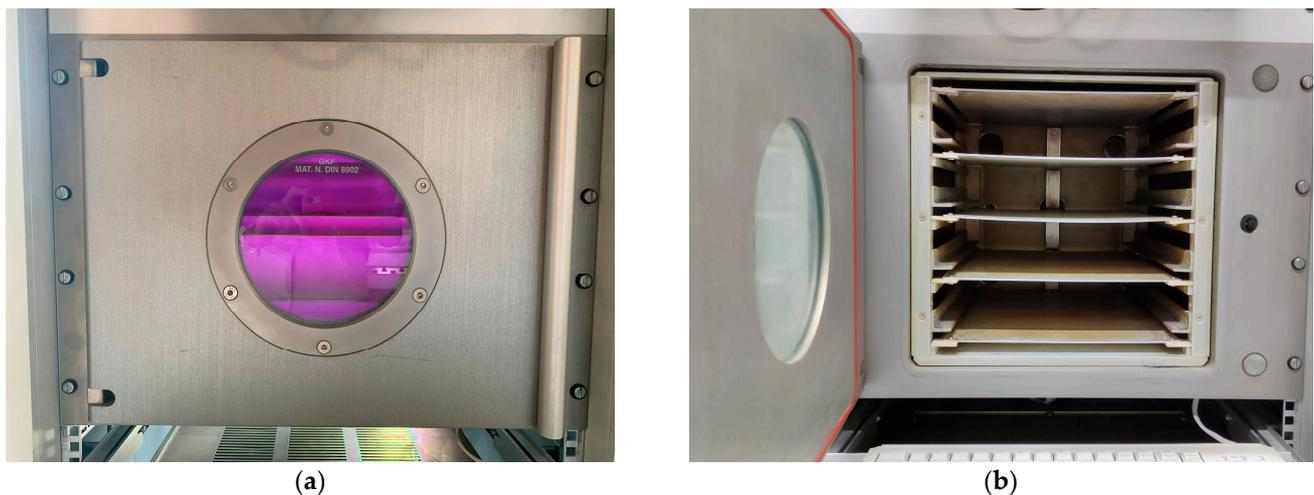
**Figure 2.** Low pressure plasma equipment (Diener Electronic GmbH). (a) Outside of the equipment, including the main screen and vacuum chamber door. (b) Vacuum chamber on the inside.
