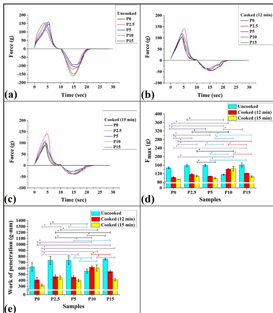
**Figure 10.** Puncture test profile of (a) uncooked, (b) 12 min cooked, and (c) 15 min cooked pasta samples; test analysis parameters: (d)  $F_{\max}$  and (e) work of penetration. (The symbol ‘\*’ on the bars shows the significant difference between the two samples at  $p < 0.05$ ).
