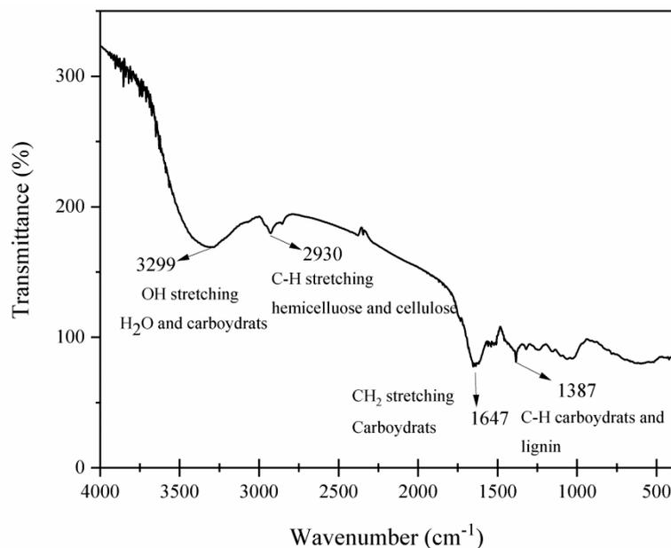
**Figure 2.** Spectrum pattern of the PBL sample.
