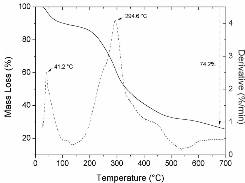
**Figure 3.** Shows the thermal behavior of freeze-dried basil leaves.
