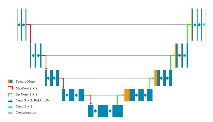
Figure 3. U-Net model architecture.
