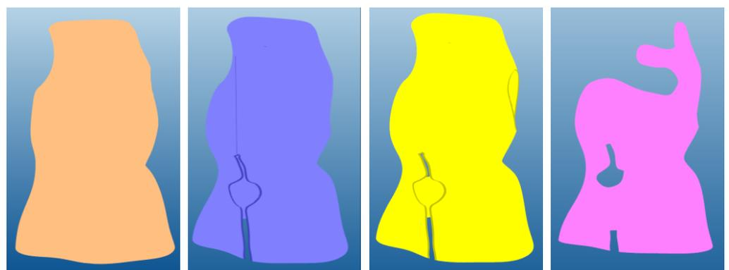
**Figure 9.** Tool paths, iterative improvement from left to right by omitting the support structures, compared to Figure 4.
