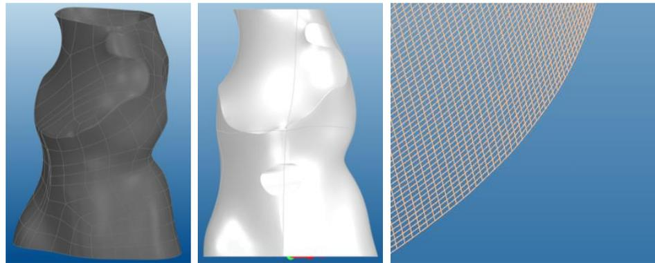
**Figure 8.** Polymesh brace (left), UV mesh (centre); details of the UV mesh (right).
