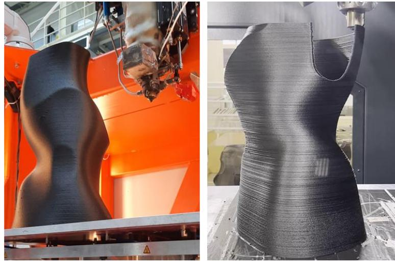
**Figure 10.** Closed orthosis with support structures at the SEAMHex 1 (left); continuous printing with cut-outs using the bypass system at the SEAMHex 2 (right).
