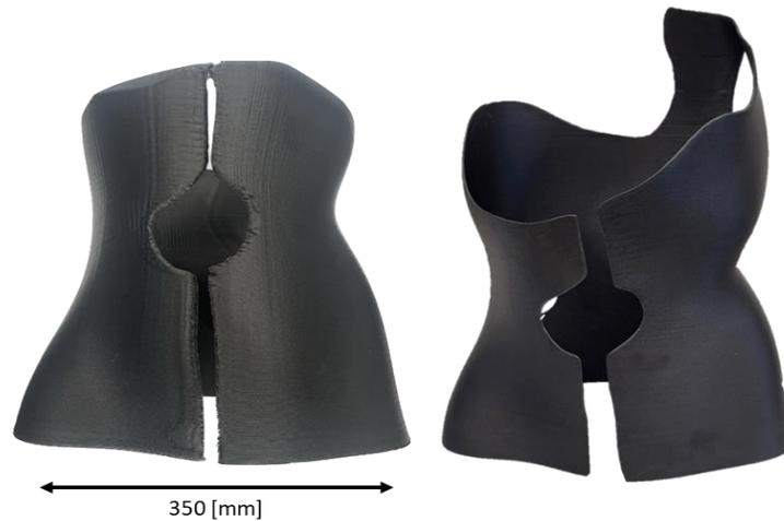
**Figure 12.** Non-post-processed print result without support structures (left); final post-processed 3D printed orthosis (right).
