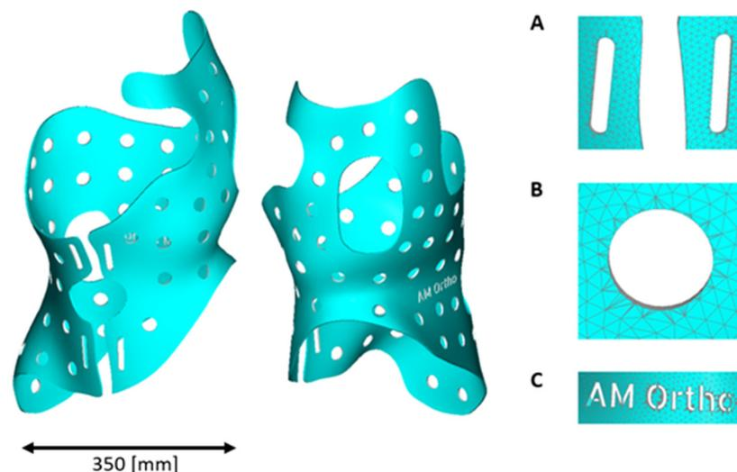
**Figure 7.** Representation of a brace with subsequent integration of pattern and functional elements such as (A) closure openings, (B) breathing patterns, or (C) letters.
