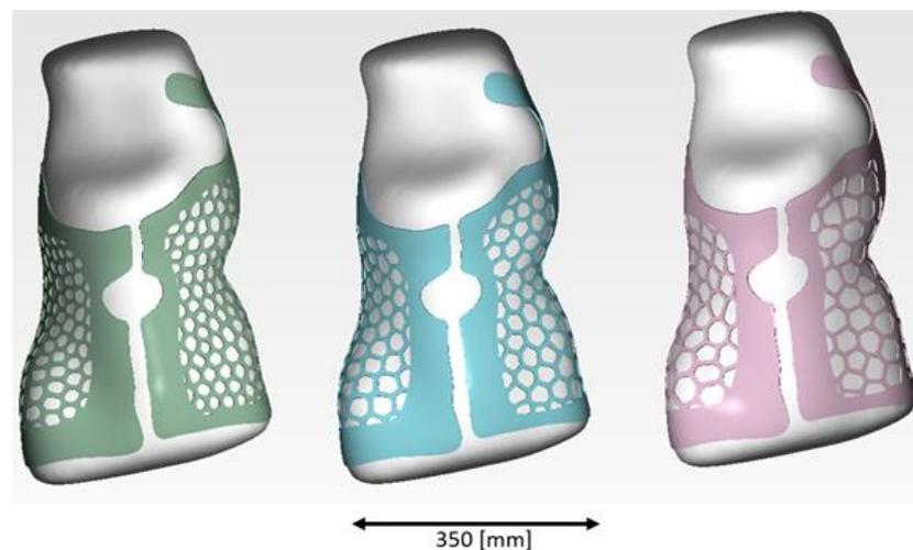
**Figure 6.** Representation of a Voronoi pattern based on a Poisson disc distribution for different discrete cell distances (parametrically adjustable) integrated into a brace volume model.
