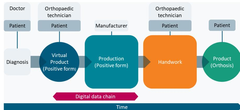
**Figure 1.** Currently established orthosis production process and data flow.
