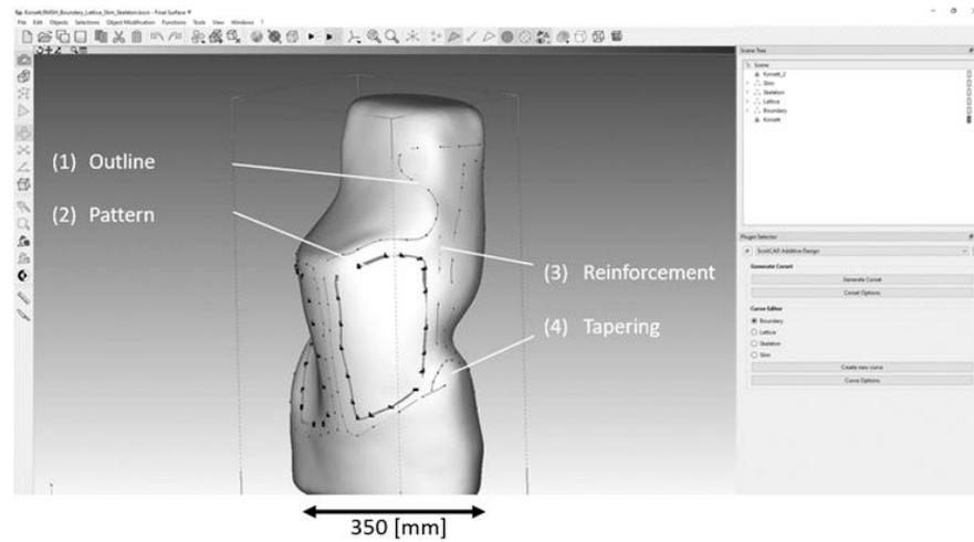
**Figure 5.** Graphical user interface (GUI) of the modelling software for orthoses and braces.
