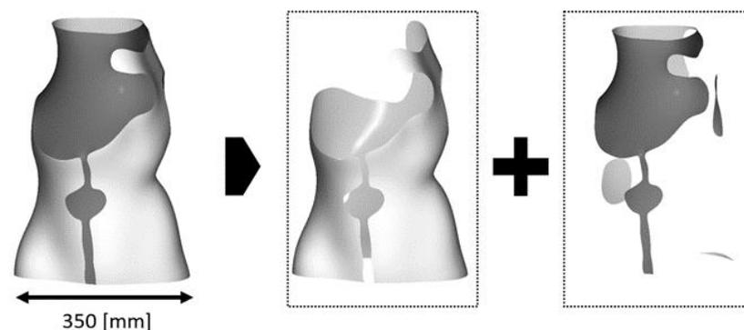
**Figure 4.** 2D middle surfaces of the orthoses, separately for the orthosis surface (light grey) and the support (dark grey).
