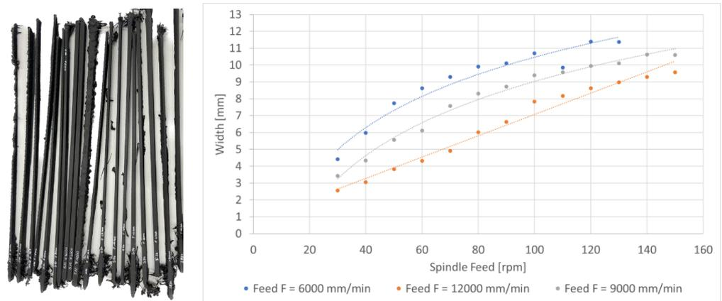
**Figure 11.** 3D-printed strips from printing tests with varying parameters using a main nozzle of 2 mm diameter and the material Akromid PA6CF40 (left); exemplary evaluation of the printing tests with regard to spindle feed, feed forward, and bead width (right).
