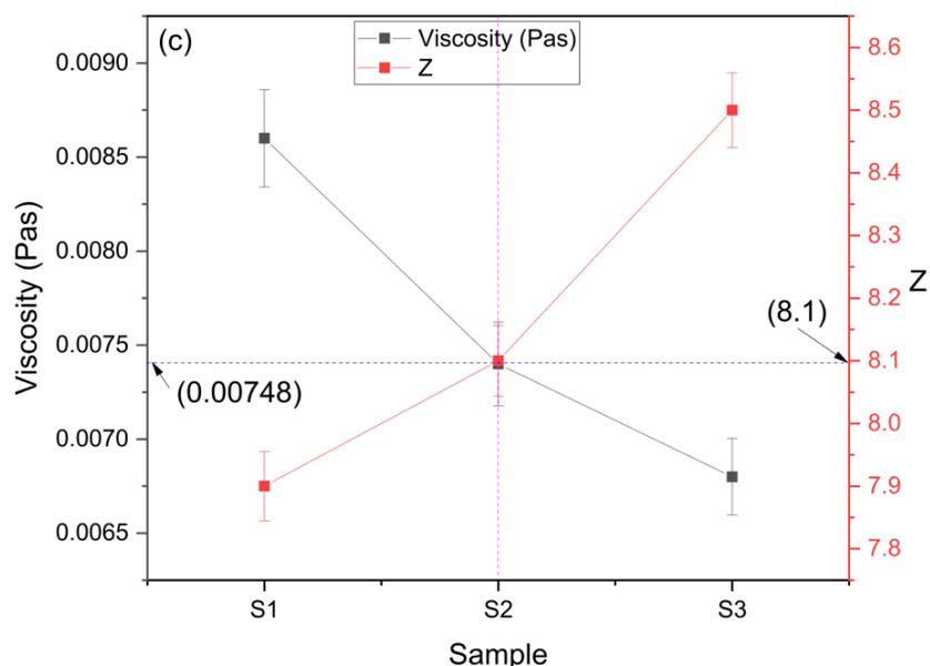
**Figure 1.** Optimization of modified CS physical properties (a) Density—Z; (b) Surface tension—Z; (c) Viscosity—Z.
