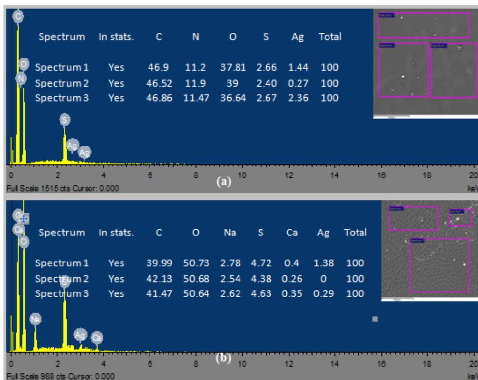
**Figure 3.** Elemental analysis at drop velocity of (a) 1.8 m/s, and (b) 2.6 m/s.
