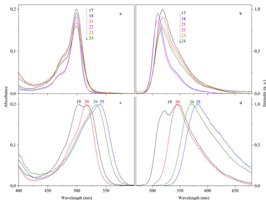
**Figure 1.** Absorption spectra (a,c) and photoluminescence (PL) (b,d) of the target BODIPY derivatives **17–20** and BODIPY triterpenoid conjugates **21–26**. T = 298 K, C =  $10^{-6}$  mol·L<sup>-1</sup> in MeOH,  $\lambda_{exc}$  = 350 nm, Fluorolog-3,  $\Delta\lambda$  = 1 nm.
