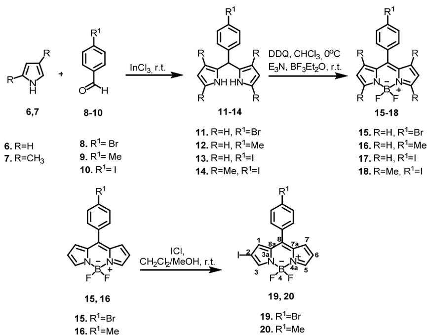
**Scheme 2.** Synthesis of *meso*-aryl-substituted derivatives boron-dipyrromethene difluoride (4,4-difluoro-4-bora-3 $\alpha$ ,4 $\alpha$ -diazas-indacene) (BODIPY) **15–20**.
