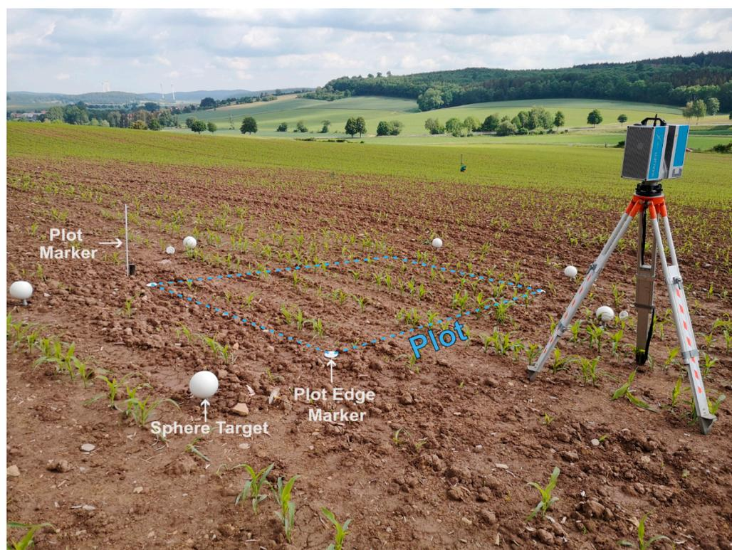
**Figure 3.** Measurement set-up during data acquisition for a scan of plot 1. The boundary of the plot is sketched in light blue.
