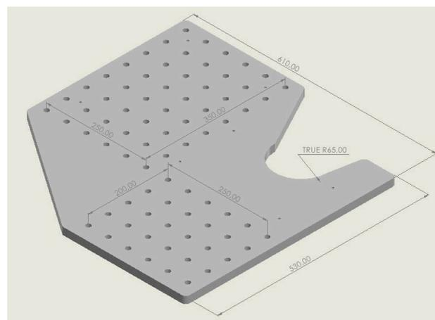
**Figure 3.** The track base and storage are designed to be adapted to the UR3e framework.
