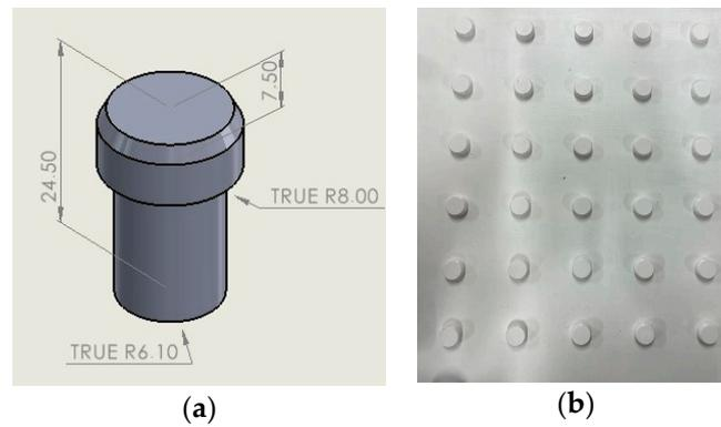
**Figure 6.** Pin: (a) pin and its measurements and (b) pins placed in the base.
