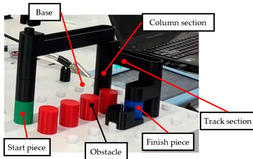
**Figure 2.** An example of a track constructed with the UR3e. The colored pieces define the path, along with the track made up of black pieces.
