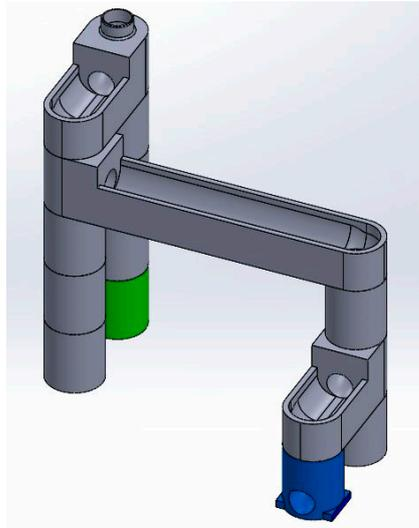
**Figure 15.** The track built with five iterations, which is the most complex type of path that UR3e can build in this framework.
