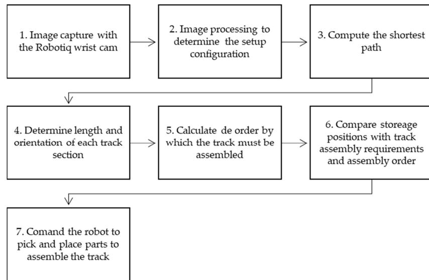
**Figure 17.** Program flowchart that enables track analysis and assembly.
