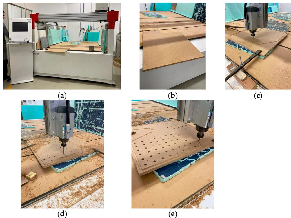
**Figure 4.** The manufacturing process of the wooden board: (a) Pronun CNC router; (b) wooden board (MDF), 650 mm × 650 mm × 18 mm; (c) drilling with a 5 mm diameter; (d) drilling with a 13 mm diameter; and (e) milling of the outer contour.
