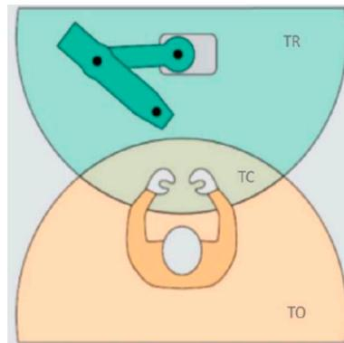
**Figure 1.** Collaborative workspace. Legend: TR-robot working space; TC-shared workspace; TO-operator workspace (adapted from [10]).
