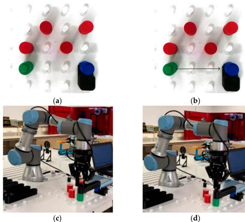
**Figure 18.** Movement sequence of Protocol 2—track with a single straight. (a) Example of piece arrangement. (b) Shortest path. (c) Assembly level 1. (d) Marble placement.
