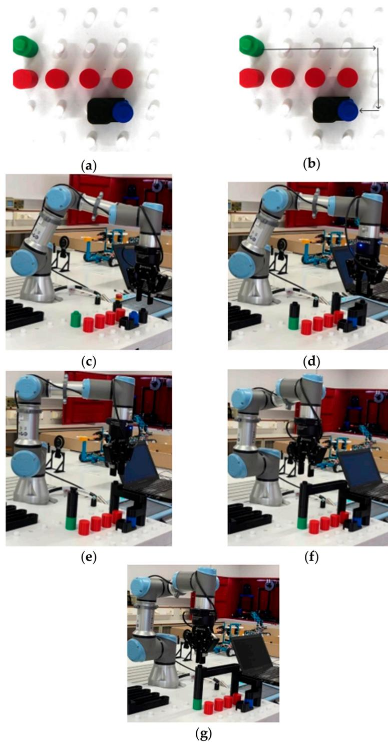
**Figure 20.** Movement sequence of Protocol 2—track with three straight sections and two curves. (a) Example of piece arrangement. (b) Shortest path. (c) Assembly level 1. (d) Assembly level 2. (e) Assembly level 3. (f) Assembly level 4. (g) Placing the marble to traverse the track.
