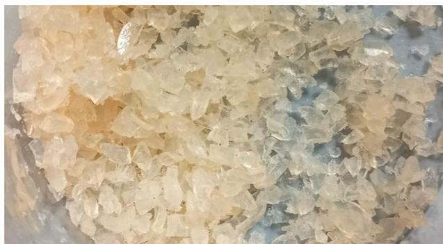
**Figure 3.** Pip–agar broken down into small fragments (before heating).
