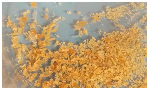
**Figure 4.** Pip-agar broken down into small fragments (after heating).
