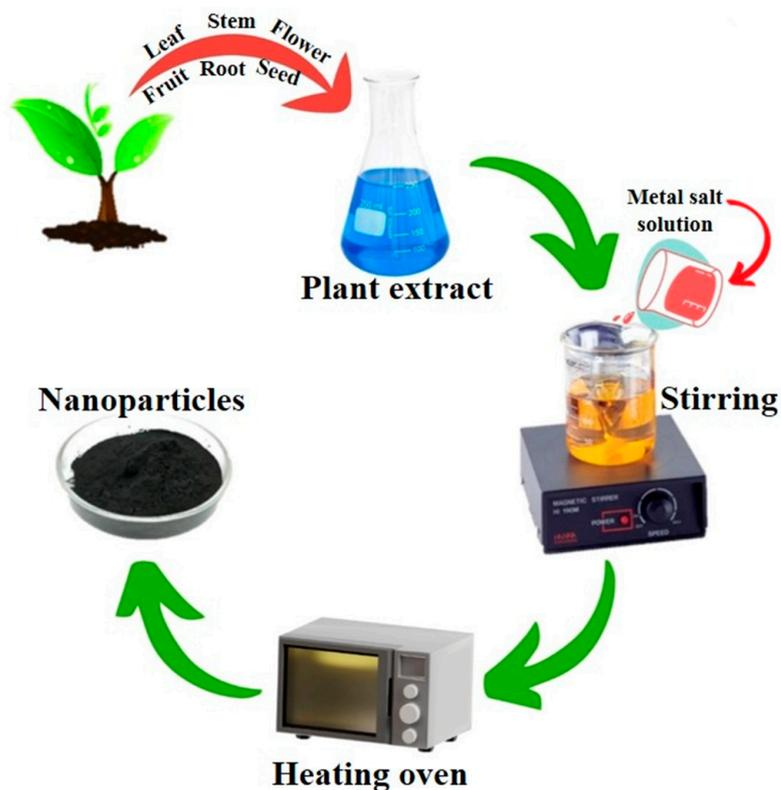
**Figure 10.** Stepwise schematic illustration for plant-mediated synthesis of Fe NPs.
