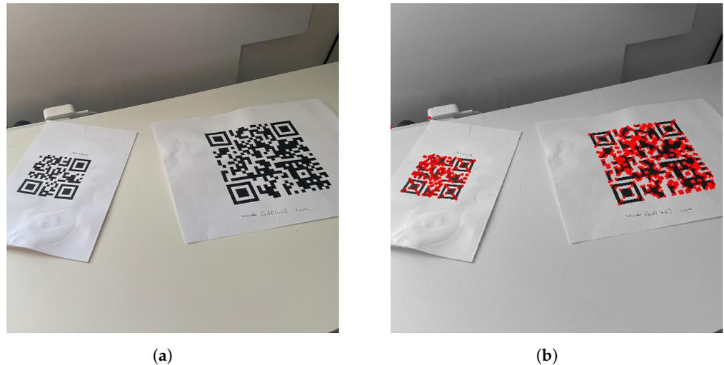
**Figure 6.** Harris corner detector can detect and pick up corners on QR codes. (a) Image of two QR codes. (b) Detected edges on two QR codes with red indicators.
