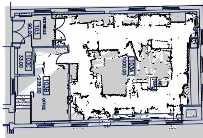
**Figure 11.** A comparison of the floor plan with the QRD LiDAR mapping.
