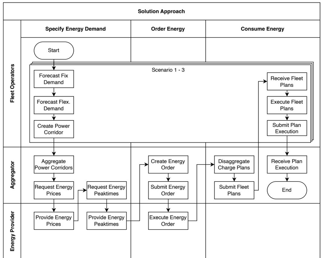
Figure 3. Flow chart of the solution approach per phase and actor of the demonstrator.
