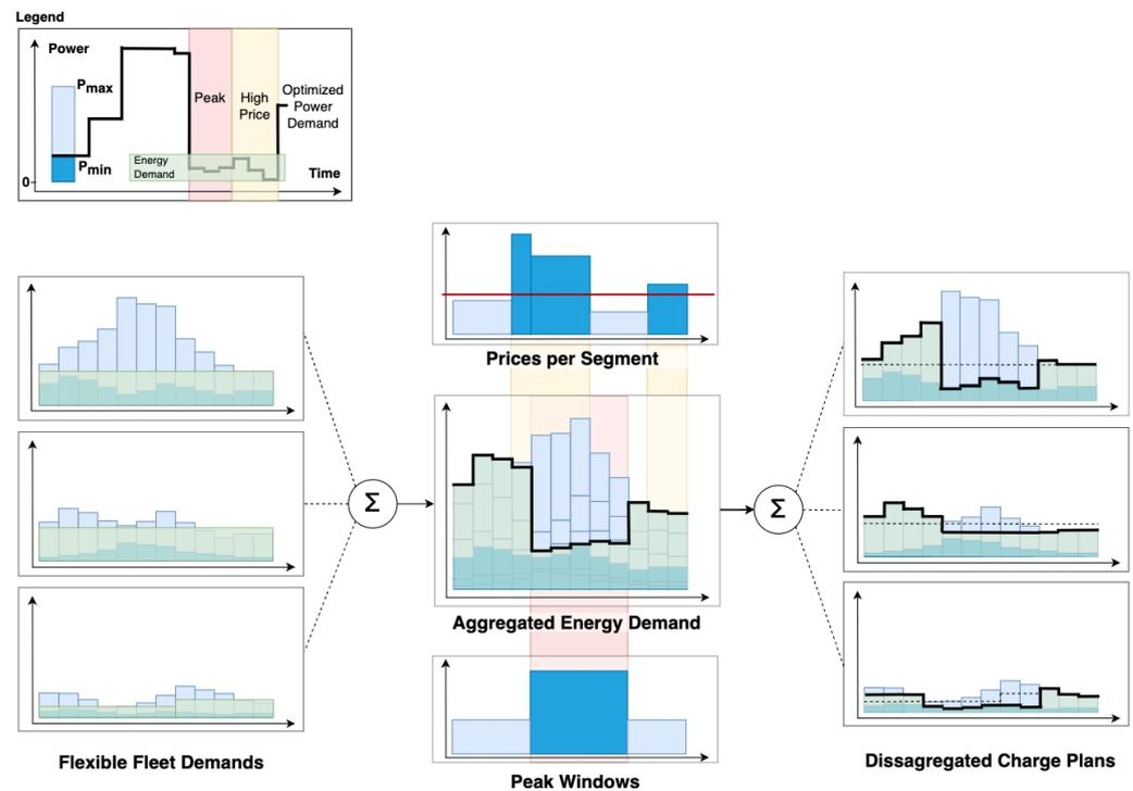
**Figure 8.** Energy aggregation process. The energy demand is aggregated to place purchasing orders, preferably at times with low prices and no peak loads. The disaggregation considers the minimum and maximum power values communicated by the fleet operators' charging systems.
