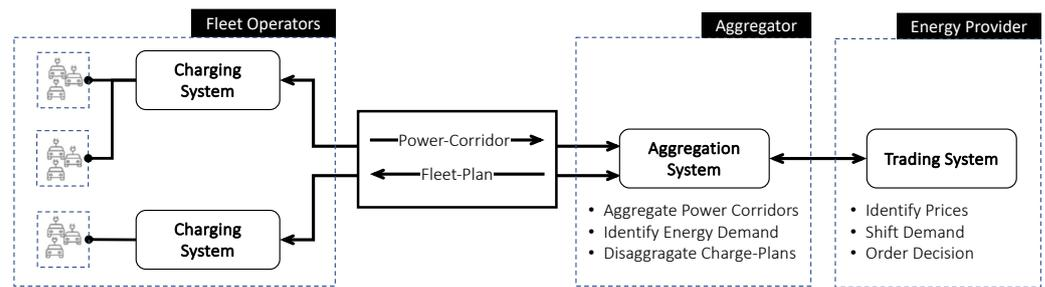
**Figure 7.** High-level architecture and main information flows between the involved roles within the demonstrator system.
