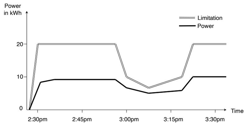
**Figure 4.** Definition of a CP charging plan based on the charging optimizer of a charging system. The CP charging plan provides the power limitation per charge point for every minute of the charging session. The actual power drawn from the EV for charging the battery is below the limitation.
