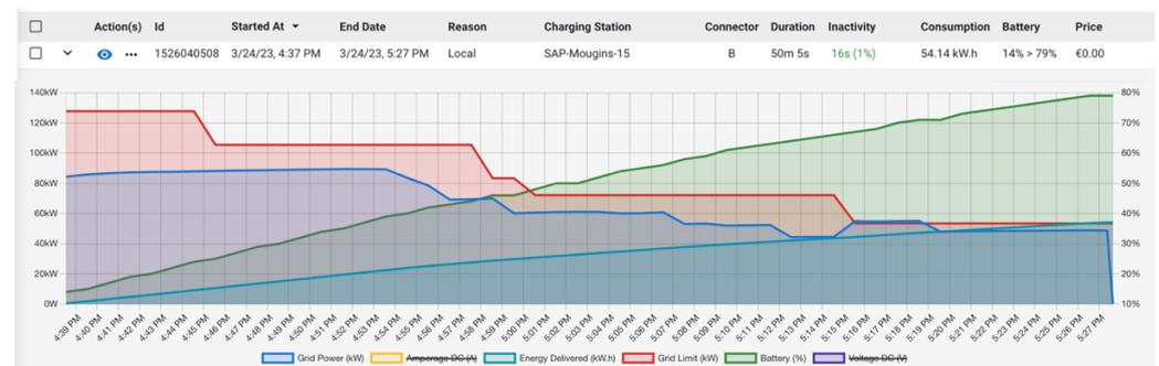
**Figure 6.** Example of a charging session in the demonstration charging system of SAP [17]. An increasing state of charge lowers the power consumption, and at 80%, the charging session ends.
