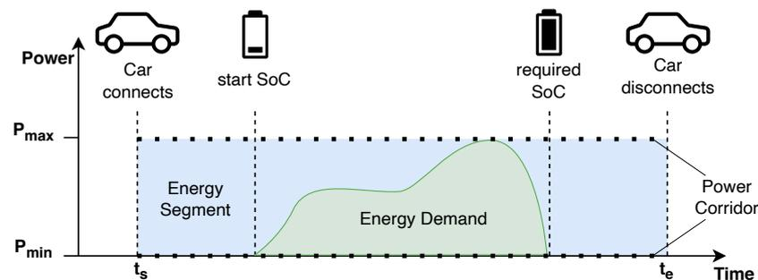
**Figure 2.** Schematic illustration of a power corridor. The power demand for charging the EV's battery starting by  $SoC_{\text{start}}$  to the required  $SoC_{\text{req}}$  level can be set between  $P_{\min}$  and  $P_{\max}$  within the time interval  $t_s$  and disconnection  $t_e$  of the EV.
