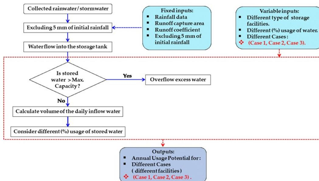
**Figure 5.** The schematic procedure of daily water inflow simulation model developed in the current study, considering the SWH facility's inputs, variable inputs, and outputs.
