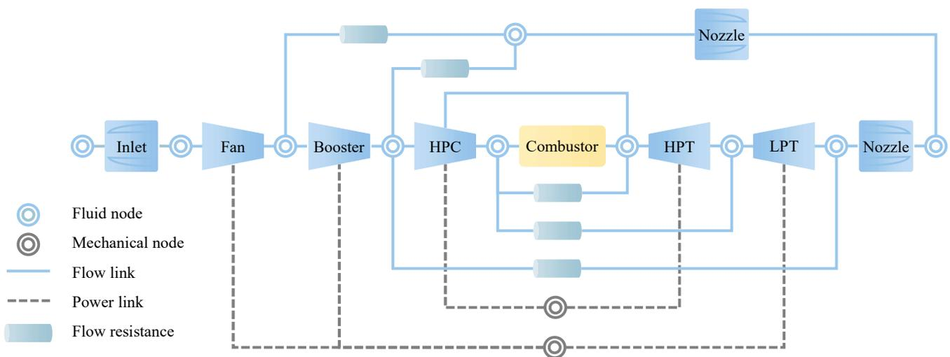
**Figure 3.** Aerodynamic-conservative network topology of the IEM.
