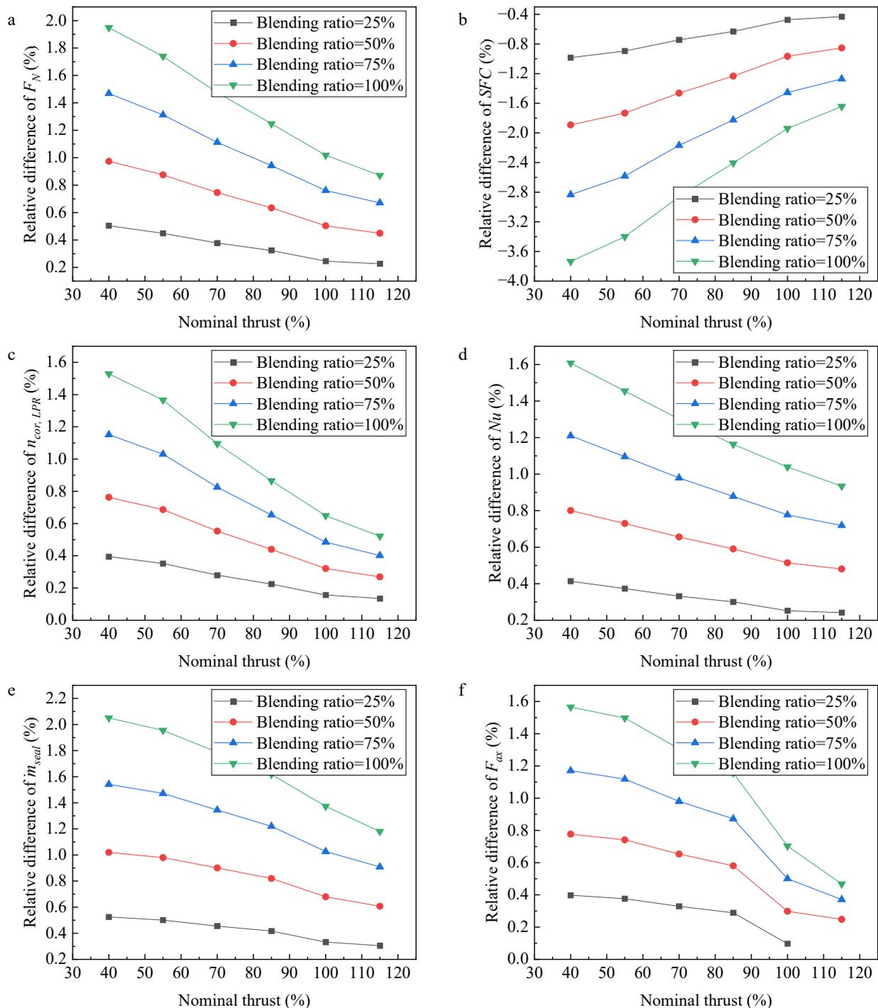
**Figure 4.** SAF's influence on (a) specific thrust; (b) specific fuel consumption; (c) turbine rotating speed; (d) turbine disk heat transfer; (e) cavity sealing air flow; (f) rotor axial load.
