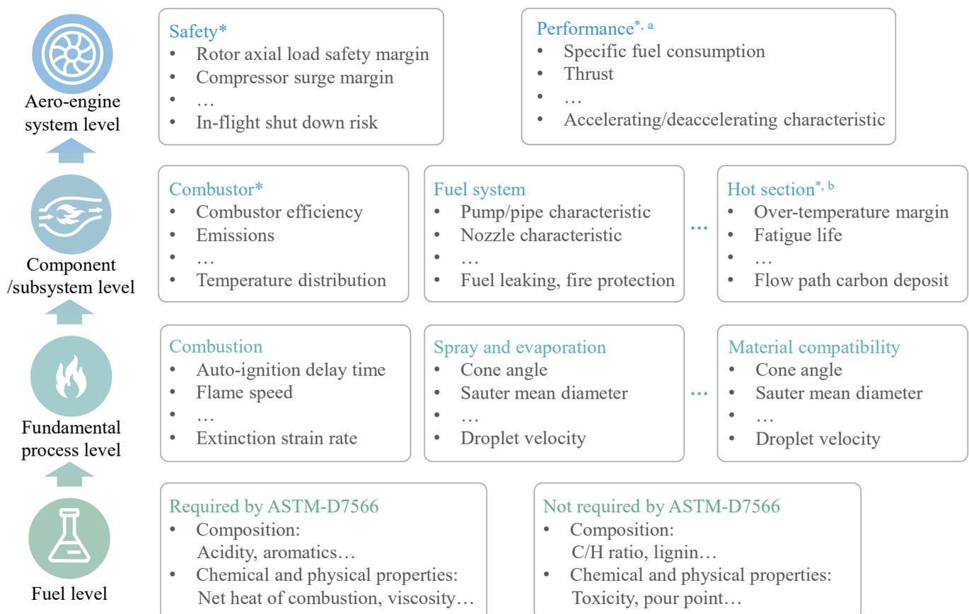
**Figure 1.** Different research levels of SAF's influences on aero-engine. \* The scope of this paper. a. Performance parameters are generally considered as SCPs in this paper, since they may influence the aircraft's survivability when encountering dangerous. b. Some component-level effects are suggested to research within the aero-engine system environment, since the component's boundary conditions are determined by the co-work point.
