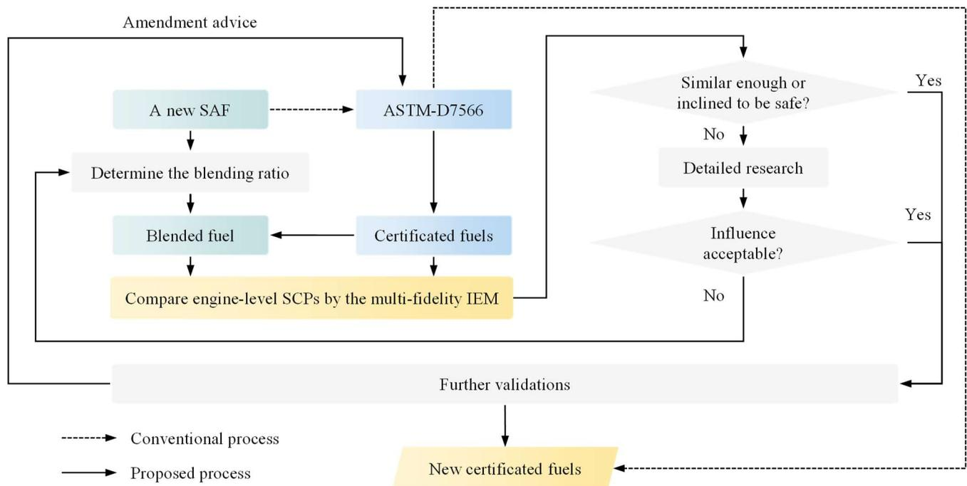
**Figure 5.** SAF's engine-level comparative safety assessment.
