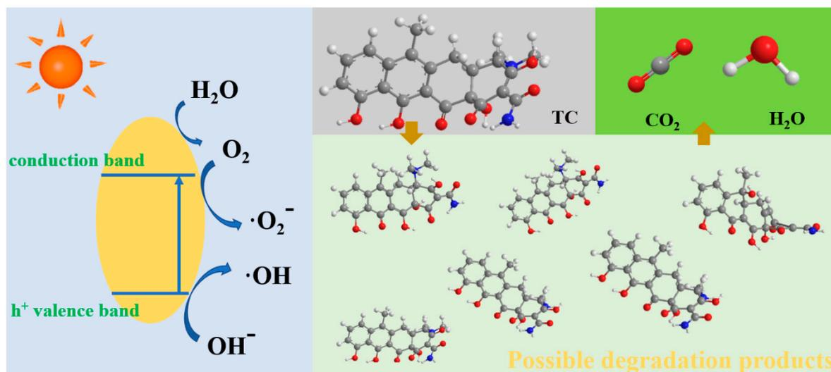
Figure 5. Mechanism of photocatalytic treatment of tetracycline antibiotics [9].
