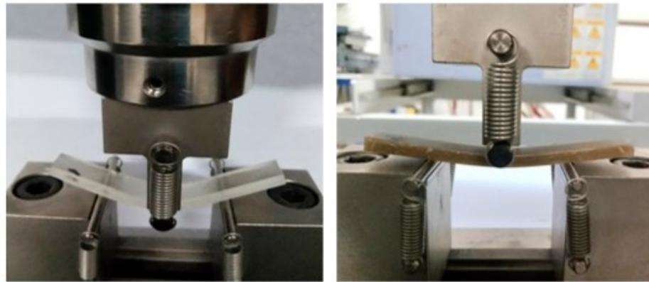
Figure 7. Flexural three-point bending test.
