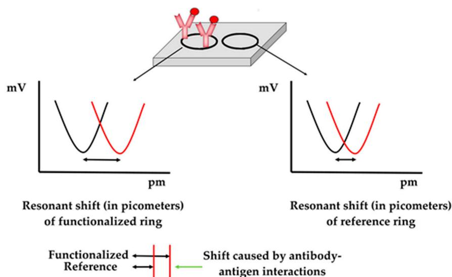
**Figure 3.** Shift calculation principle. The black lines in the plot represent the state of the sensor (minimum) prior the introduction of the sample, whereas the red lines represent the state of the sensor (minimum) after introducing the samples.
