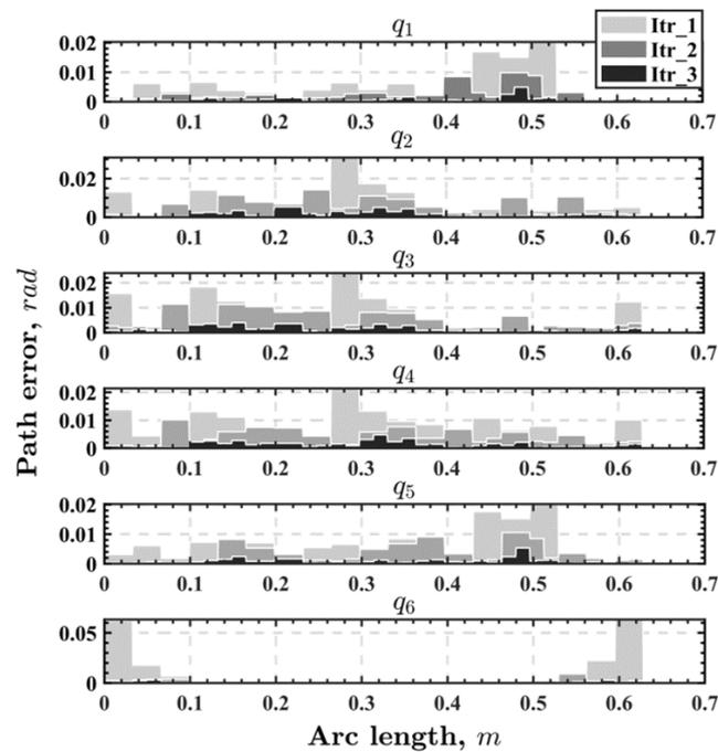
Figure 5. Path discretization error reduction in each iteration.
