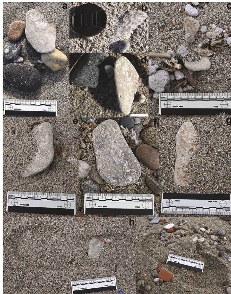
**Figure 2.** Fragments of ACM outcropping in the beaches of the study area (a–i). Fragments appear with well-rounded sub-elongate shapes and surface ornamentation (b). ACMs are partially covered by sands (a–e,g,i). (h,i) Boot prints on the sand showing the human–environmental interactions. The two fragments of ACM were trampled by humans, enhancing their fracture and the transfer of the fibers from the cement to humans and the environment. Source: Authors.
