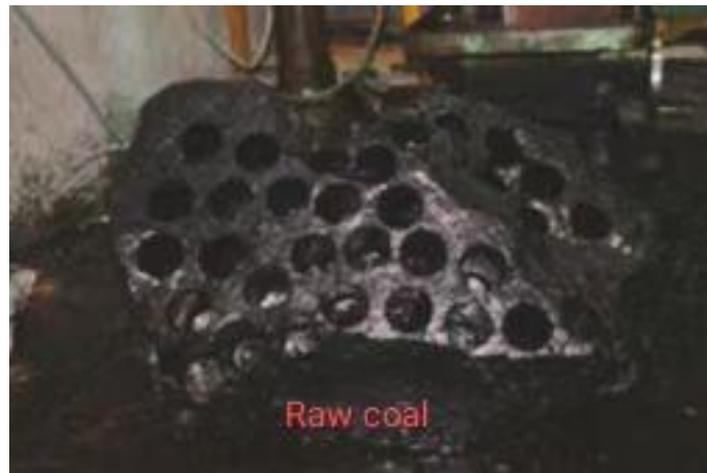
Figure 4. Drilling of raw coal test pieces.
