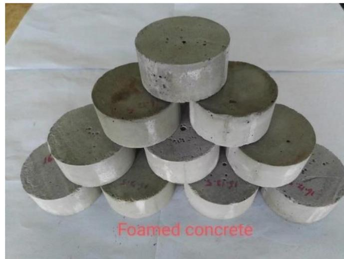
**Figure 6.** Foam concrete specimen.
