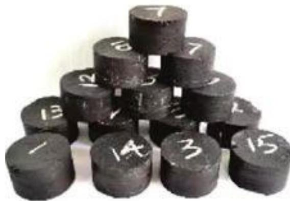
Figure 5. Raw coal test pieces.
