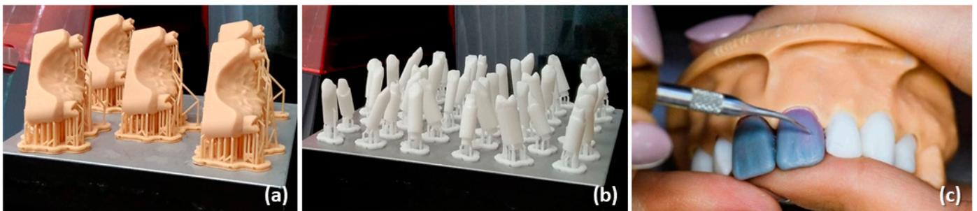
**Figure 1.** Dental model and stumps: (a) printed dental models, (b) printed dental stumps, (c) work on the assembled dental model.
