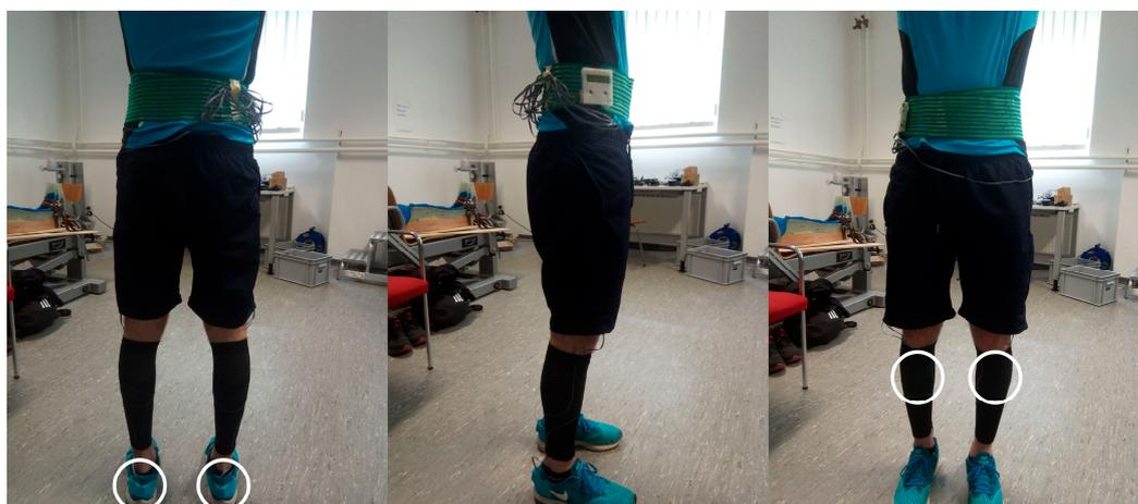
**Figure 1.** Full IMU setup. White circles indicate the positions of the placed sensors used for analysis.
