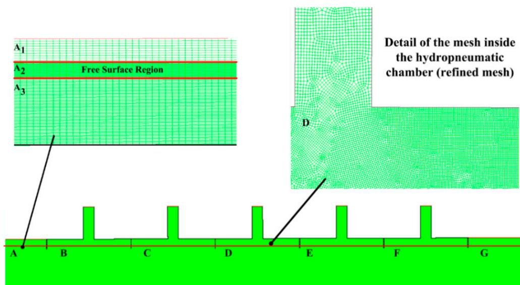
**Figure 4.** Numerical bidimensional mesh of the computational domain.
