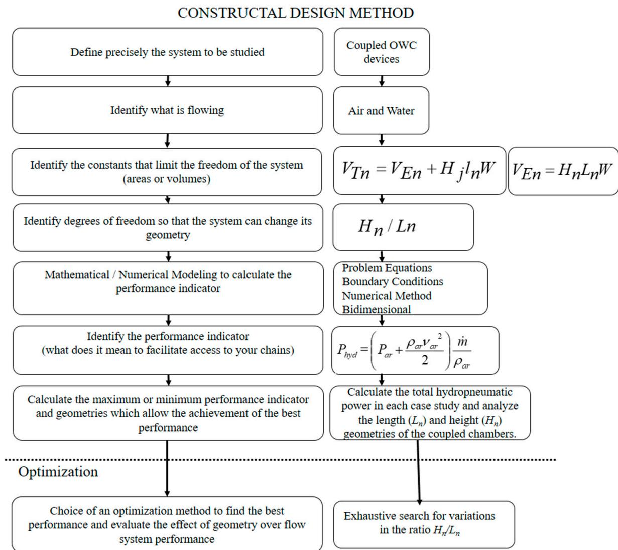
Figure 2. Execution steps of the Constructal Design method.
