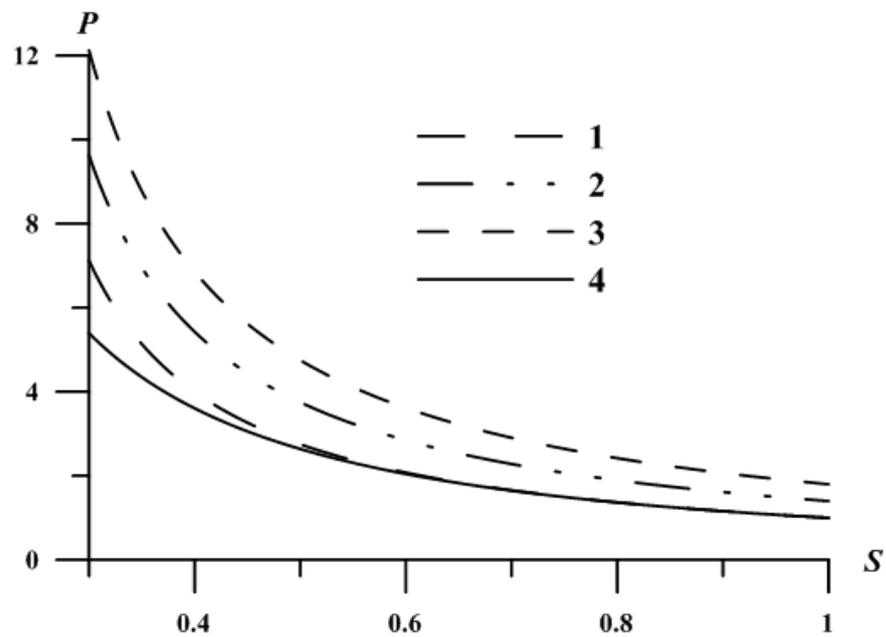
**Figure 2.** Effect of heat release,  $Q$ , on the Hugoniot curve at  $M = 0$ ; 1— $Q = 0$ ; 2— $Q = 2$ ; 3— $Q = 4$ ; 4—the Poisson isentrope.
