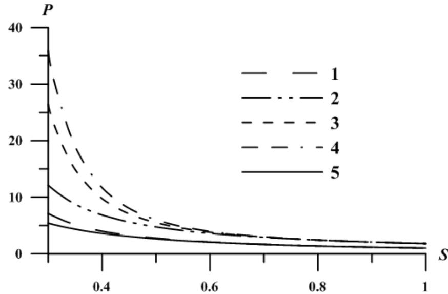
**Figure 4.** Effect of  $Q$  and  $M$  on the Hugoniot curve: 1— $M = 0$ ,  $Q = 0$ ; 2— $M = 0$ ,  $Q = 4$ ; 3— $M = 3$ ,  $Q = 4$ ; 4— $M = 5$ ,  $Q = 4$ ; 5—the Poisson isentrope.
