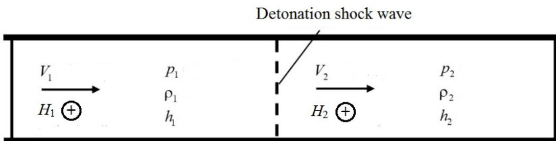
Figure 1. Schematic outline of the shock wave geometry.
