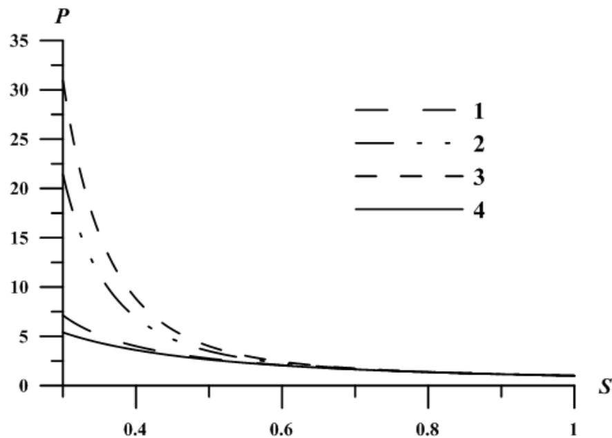
**Figure 3.** Effect of intensity of the magnetic field,  $M$ , on the Hugoniot curve at  $Q = 0$ ; 1— $M = 0$ ; 2— $M = 3$ ; 3— $M = 5$ ; 4—the Poisson isentrope.
