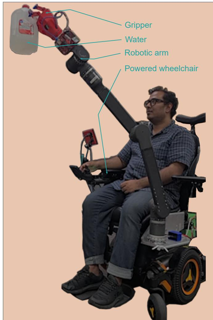
Figure 10. Load testing with mR2A robot.
