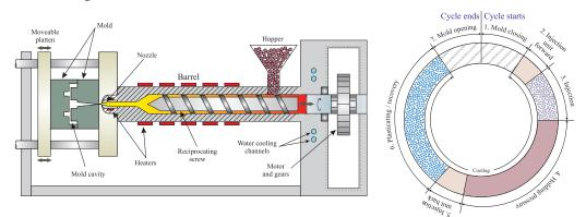
Figure 1. A schematic of injection molding machine and a molding production cycle.
