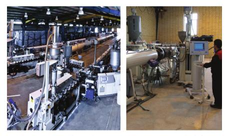
Figure 11. Injection molding and extrusion machines in Semnan Polyethylene Pipe and Fitting Co.
