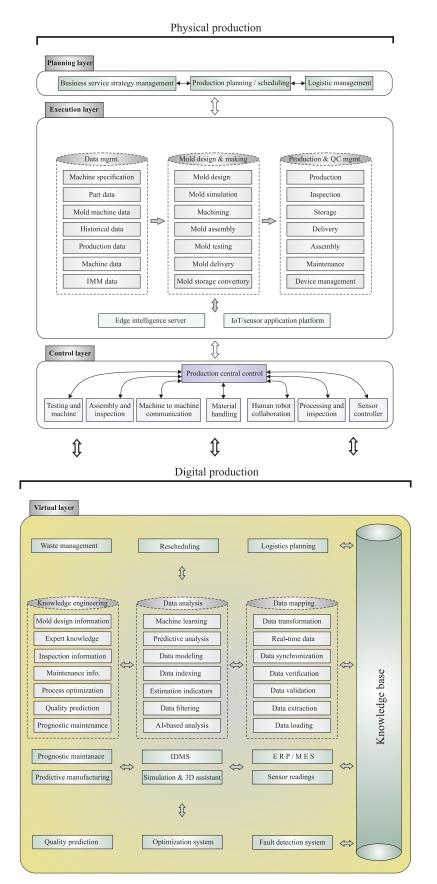
Figure 4. Knowledge-based framework of DT model for smart injection molding.
