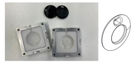
Figure 8. Fabricated 3D-printed mold for production of the chip key.
