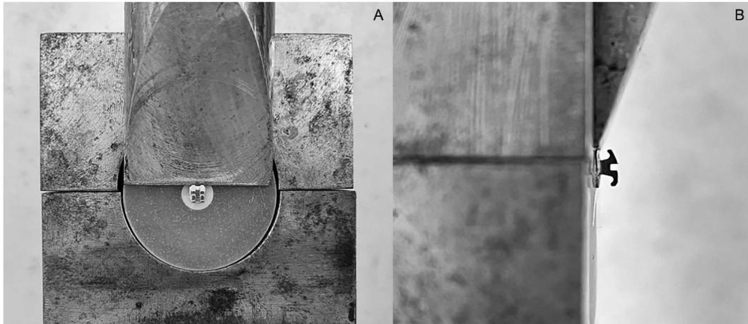
**Figure 3.** (A,B) Shear bond strength test with the universal testing machine.
