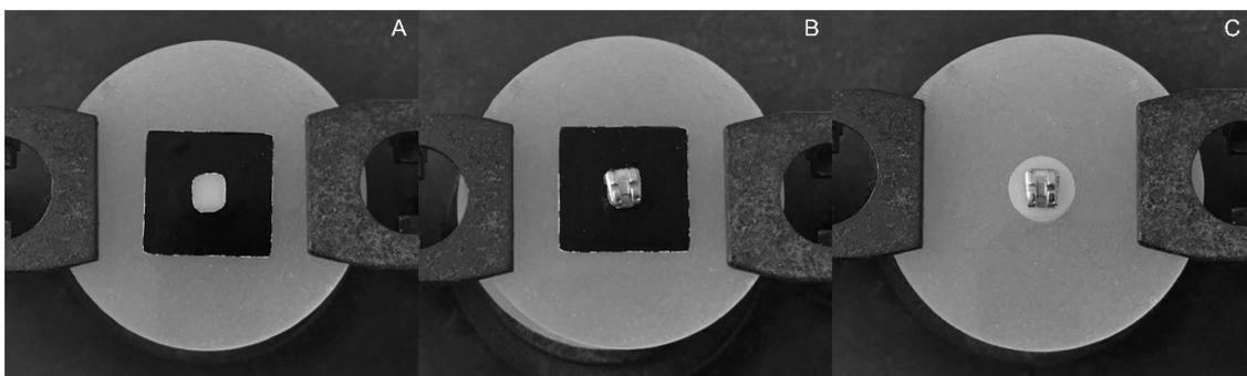
**Figure 2.** Bracket bonding procedure. (A) The bonding area was defined by a custom-made waterproof sticker. (B) The bracket was placed onto the zirconia surface. (C) After light-curing, the sticker was peeled off.
