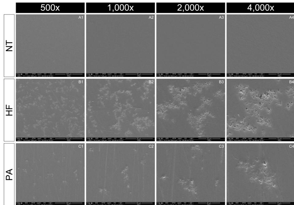
**Figure 5.** Zirconia surface topography under scanning electron microscopy at (1) 500×; (2) 1000×; (3) 2000×; and (4) 4000× magnification. (A) Specimen had no surface treatment (NT). (B) Specimen was etched with 4% hydrofluoric etchant (HF). (C) Specimen was etched with 37% phosphoric etchant (PA).
