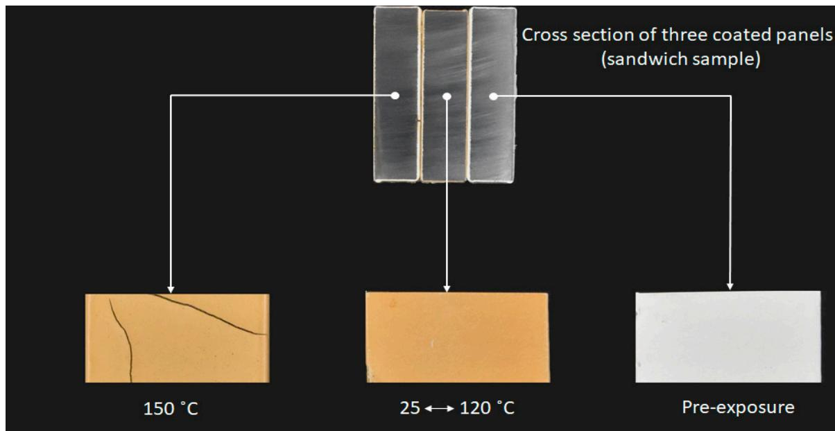
**Figure 3.** Arrangement of the three coated panels used for ToF-SIMS measurements.
