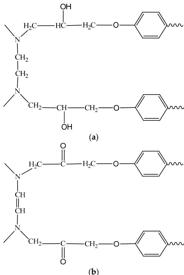
**Figure 13.** Chemical structures produced during the resin curing reaction between DGEBA and EDA hardener (a) before and (b) after heat exposure [28].
