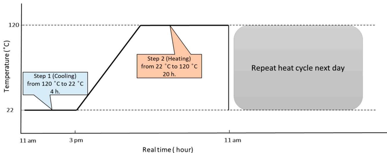
**Figure 1.** Dry thermal cycling profile (temperature vs. time).
