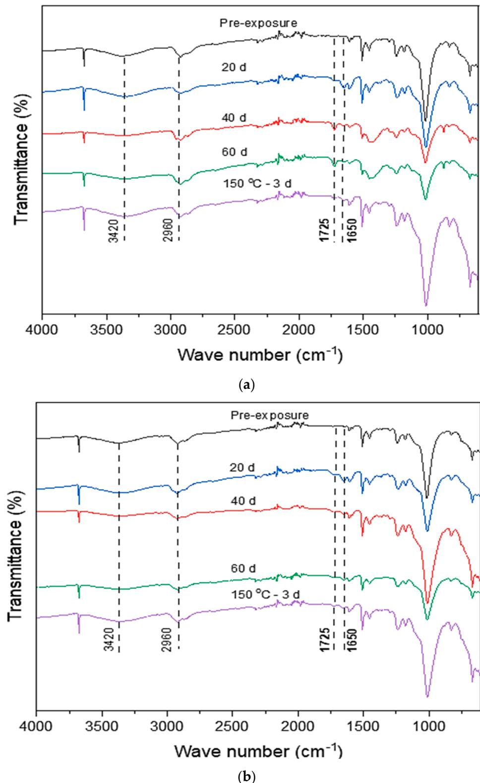
**Figure 11.** FTIR spectra phenolic epoxy coatings before and after heat treatment to a maximum of 120 °C under (a) cyclic or (b) isothermal.
