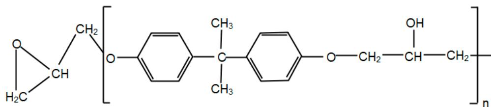
**Figure 12.** Chemical structure of DGEBA as a typical resin.
