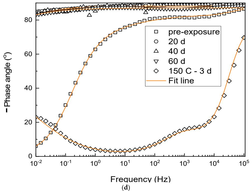
**Figure 7.** Bode plots of phenolic-epoxy-coated steel samples after immersion in 3.5 wt% NaCl solution: (a,b) cycled and (c,d) isothermal heat treatment (120 °C maximum temperature).
