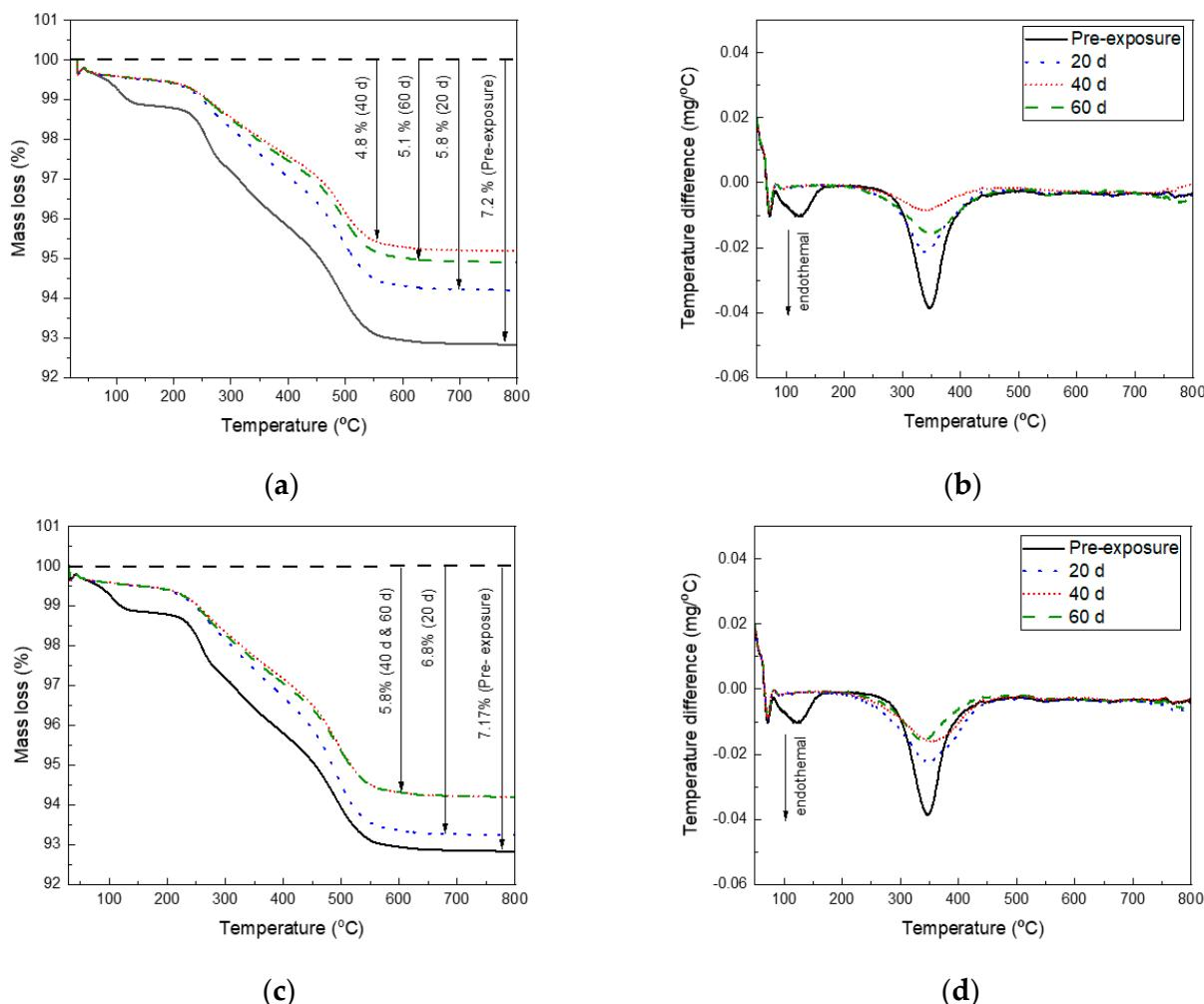
**Figure 9.** (a,c) TGA and (b,d) DTGA curves measured in air for phenolic-epoxy heat treated to a maximum of 120 °C under (a,b) isothermal or (c,d) cyclic conditions.
