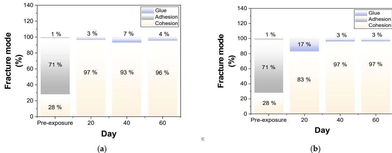
**Figure 5.** Area fractions of the failure modes of (a) isothermal and (b) cycled samples after pull-off adhesion tests.
