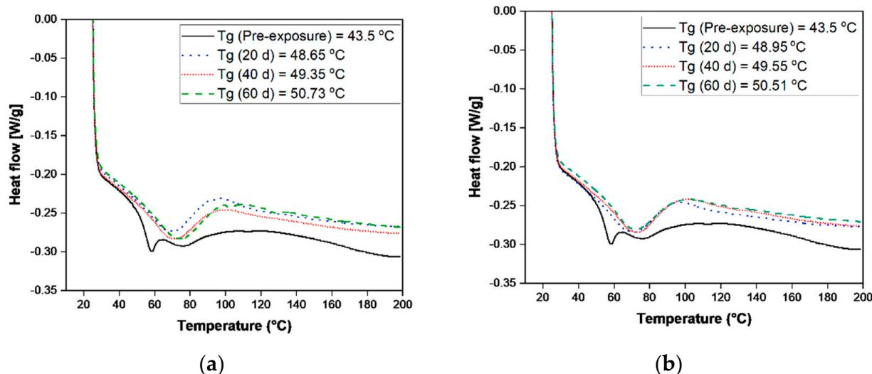
**Figure 10.** DSC curves used to determine the  $T_g$  values of phenolic epoxy coatings heat treated to a maximum of 120 °C under (a) isothermal or (b) cyclic conditions.
