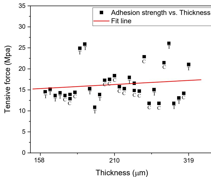
**Figure 4.** Pull-off adhesive strength as a function of the coating thickness for isothermal (C) and cycled (T) samples.
