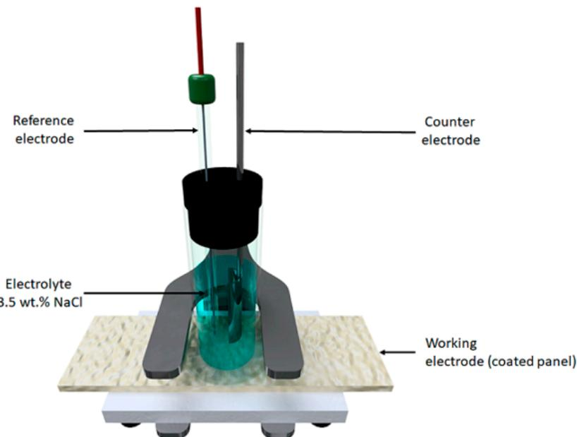
**Figure 2.** Schematic of the electrochemical cell used for testing the epoxy-coated metal sheets.
