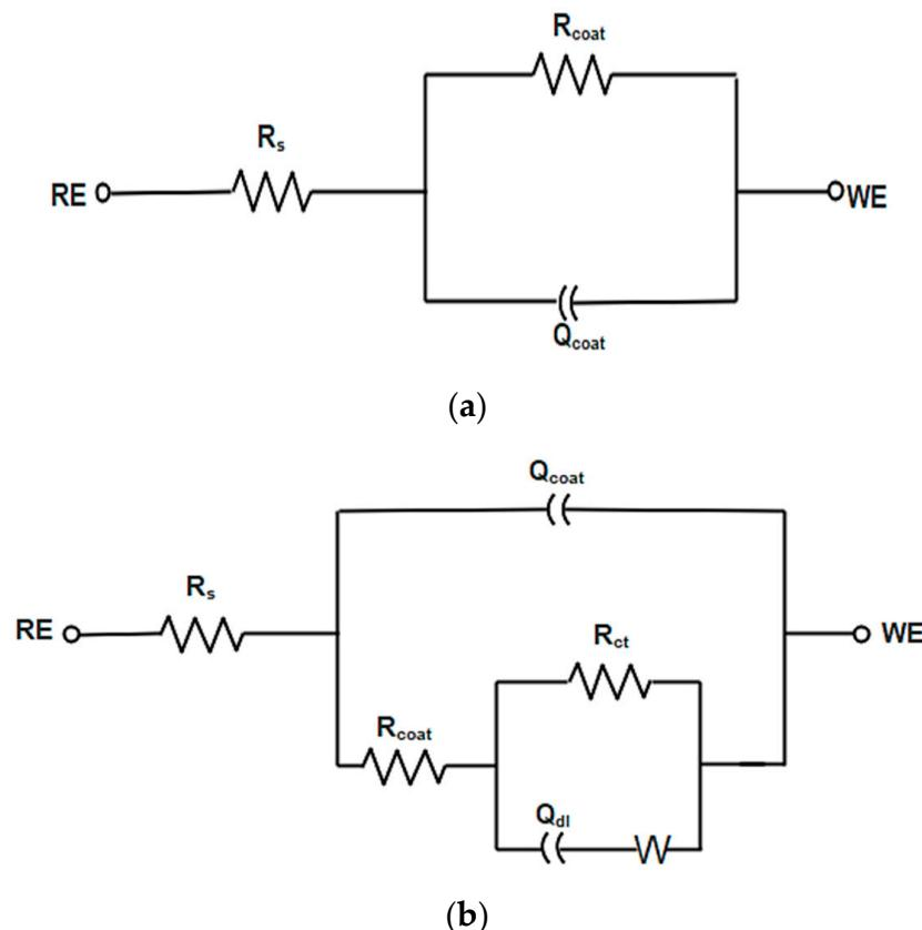
**Figure 8.** Equivalent circuits used to fit the impedance curves obtained for (a) all coated metal samples other than (b) the 150 °C isothermal sample (to account for cracks in the coating).
