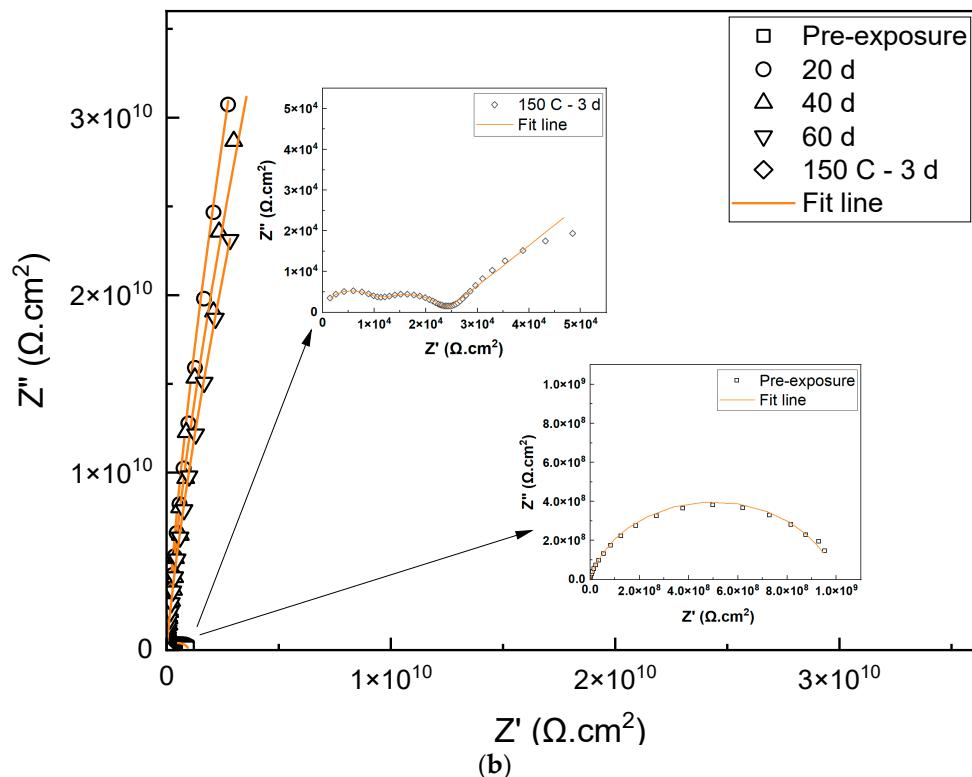
**Figure 6.** Nyquist plots of phenolic-epoxy-coated steel samples after immersion in 3.5 wt% NaCl solution: (a) cycled and (b) isothermal heat treatment (120 °C maximum temperature).
