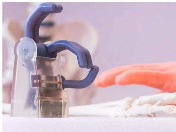
**Figure 1.** First “Iron Hand” of Götz von Berlichingen, a 3D-printed polymer replica. The replica was printed by a 3D multi-material printer, the Stratasys J750, that allows for the production of transparent components, offering insights into the mechanics of the hand. Picture credits: Offenburg University, Germany.
