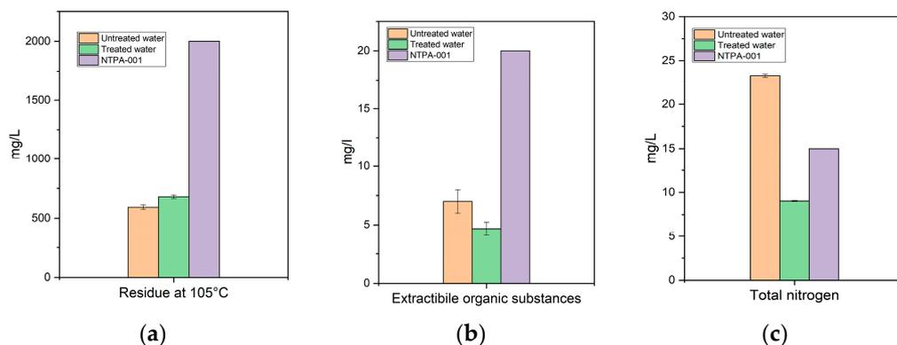
**Figure 3.** Residues at  $105^\circ\text{C}$  (a), extractible organic substances (b), total nitrogen (c), determined for initial samples from untreated water, samples after bioaugmentation treatment, and maximum threshold values.
