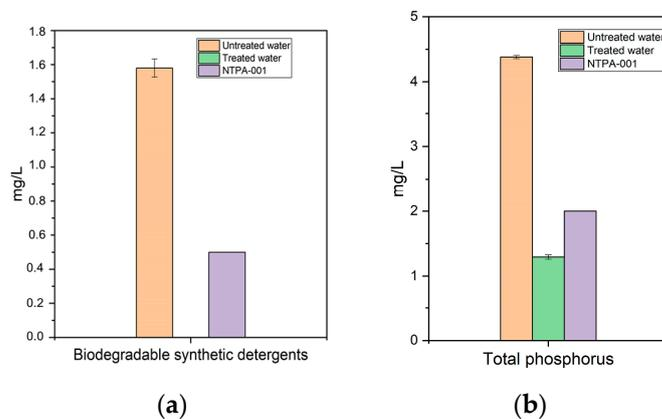
**Figure 4.** Biodegradable synthetic detergents (a), and total phosphorus (b), determined for initial samples from untreated water, samples after bioaugmentation treatment, and maximum threshold values.
