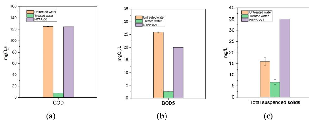
**Figure 2.** Chemical oxygen demand (COD, a), biochemical oxygen demand (BOD5, b), total suspended solid (c), determined for initial samples from untreated water, samples after bioaugmentation treatment, and maximum threshold values.
