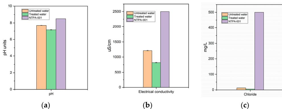
**Figure 1.** pH (a), electrical conductivity (b), and chloride values (c), determined for initial samples from untreated water, samples after bioaugmentation treatment, and maximum threshold values.
