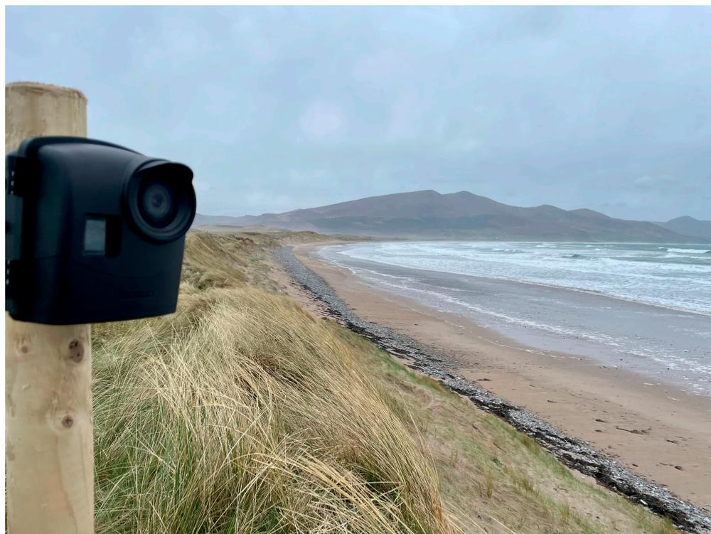
**Figure 4.** Photo of Brinno TLC2000 Camera 1 deployed in the field.
