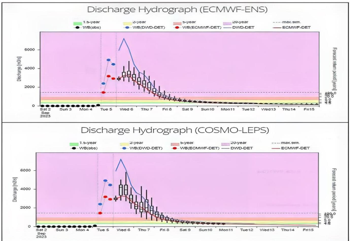
Figure 1. EFAS chain hydrograph for the hydrological section of Larissa, Pineios River [17].
