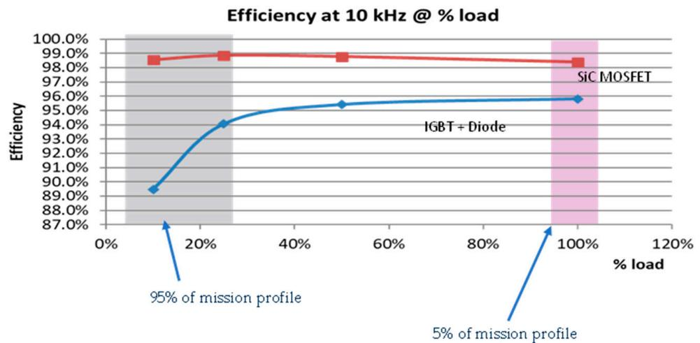
**Figure 6.** Inverter efficiency, defined as  $P_{out}/(P_{out} + P_{loss})$  for the 210 kW inverter. % load is the inverter’s output power with respect to its maximum value.
