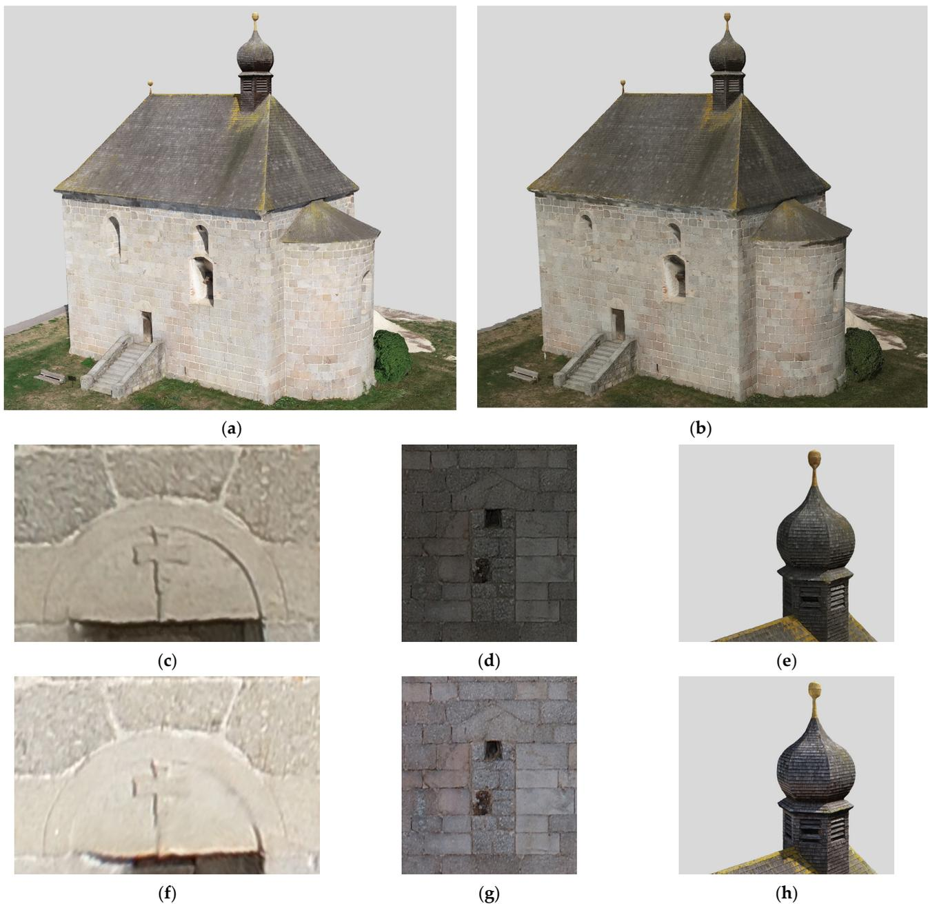
**Figure 4.** Comparison of the resulting 3D models of (a) DJI P4RTK, and (b) DJI M300 with Zenmuse P1. Both views from southeast. Detailed views taken from Zenmuse P1 result (c–e) and P4RTK (f–h): (c,f) medieval relief with a cross at the semi-circular entrance arch, (d,g) bricked-up Romanesque high entrance at western wall, and (e,h) missing slat in belfry of ridge turret. Partly, the difference in camera resolution can be observed.
