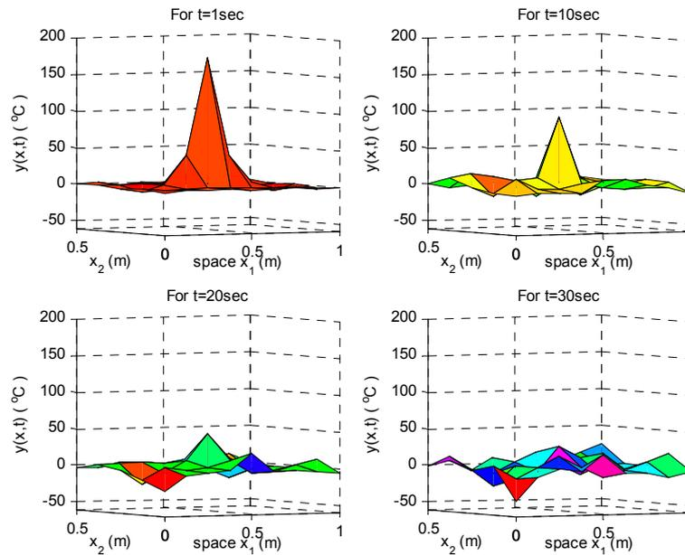
**Figure 2.** The temperature distribution  $y(x, t)$  of the heat transfer system given in Equation (71) at  $t = 1, 10, 30$  and  $50$  s. Due to the diffusion term  $\kappa \nabla^2 y(x, t)$ , the temperature of heat system will be uniformly distributed gradually to increase the system entropy.
