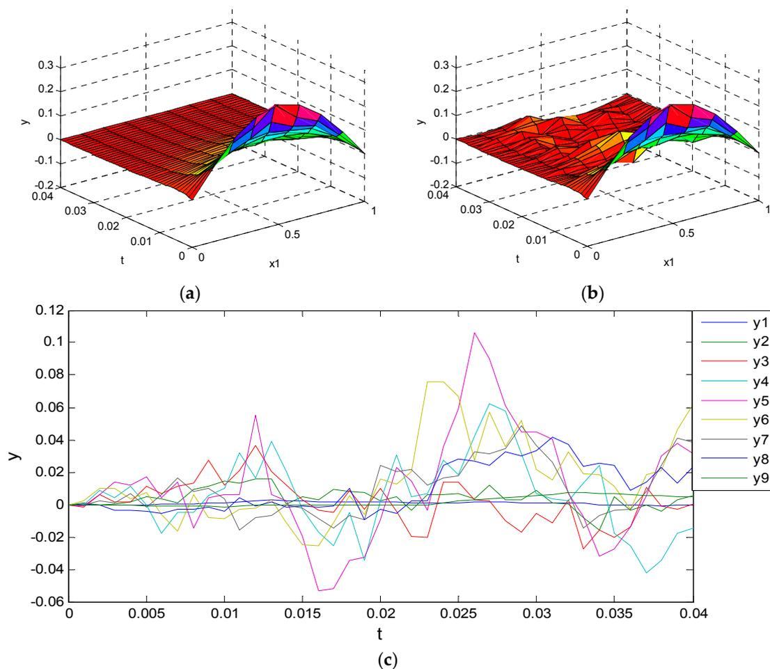
**Figure 5.** (a) Spatial-time profiles of the real biochemical system in Equation (74); (b) Spatial-time profiles of the approximated system in Equation (66) based on the finite difference scheme and global linearization technique; (c) The error between the real biochemical system in Equation (74) and the approximated system in Equation (66). Obviously, the approximated system in Equation (66) could approximate the real system in Equation (74) quite well.
