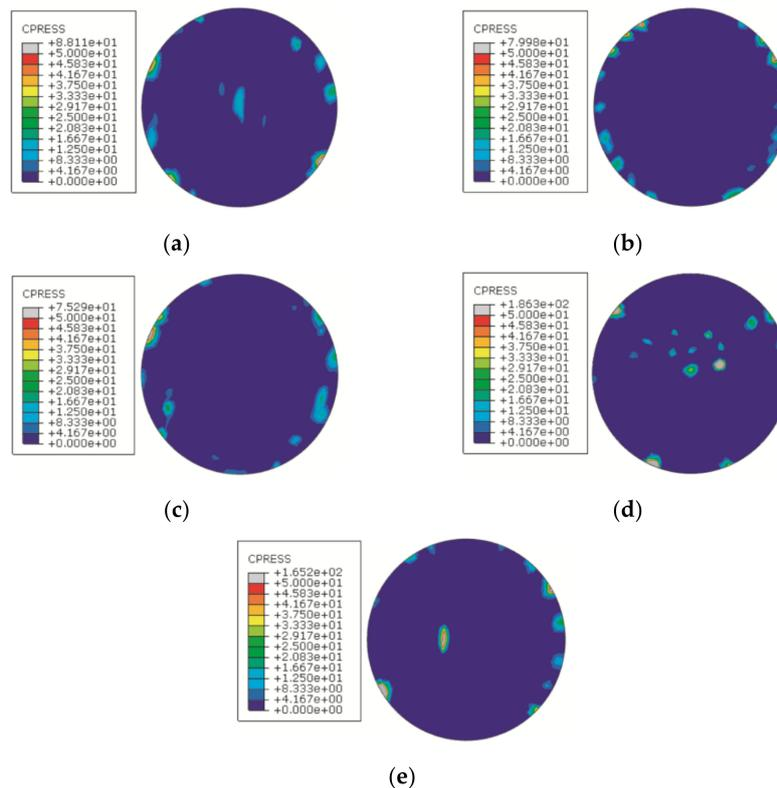
Figure 3. Contact pressure distribution contours of five samples. (a) Group 1; (b) Group 2; (c) Group 3; (d) Group 4; (e) Group 5.
