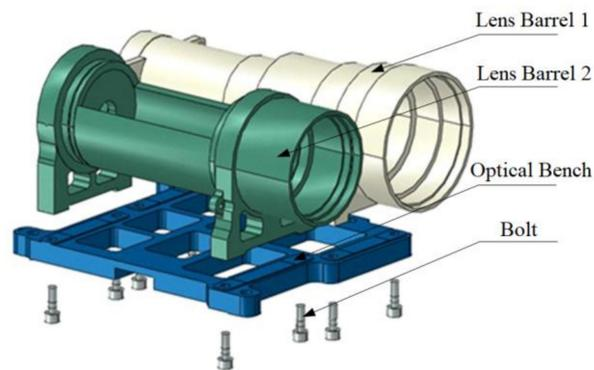
**Figure 7.** Assembly schematic of the precision optical lens.
