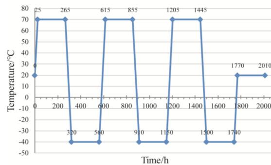
**Figure 5.** Temperature cycling curve used in experiment.
