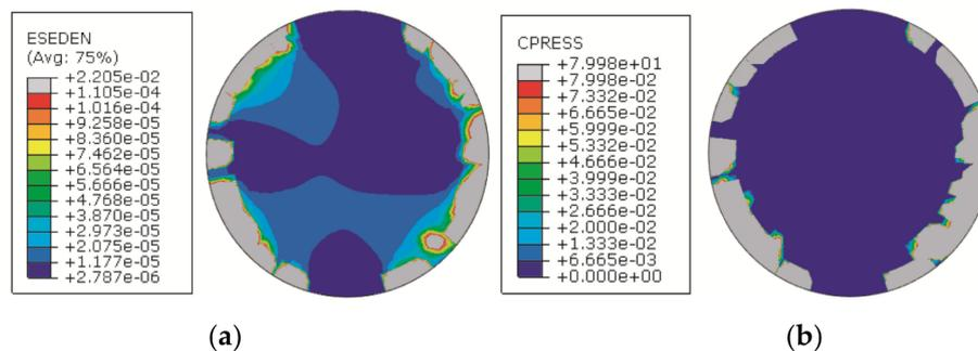
**Figure 10.** Comparison between the contact pressure and strain-energy contours. (a) Strain energy density contour; (b) contact pressure contour.
