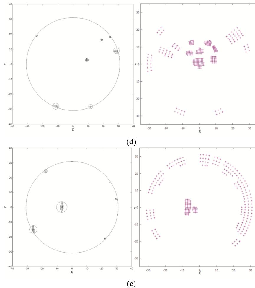
**Figure 4.** Comparison between the convex hull search results and the actual contact area. (a) Group 1; (b) Group 2; (c) Group 3; (d) Group 4; (e) Group 5.
