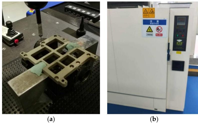
**Figure 9.** Experimental setup: (a) Coordinate measuring machine and (b) Constant-temperature test chamber.
