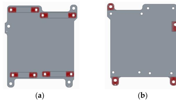
**Figure 8.** Assembly surface of optical holder: (a) Assembly surface with lens barrels and (b) Assembly surface with assembly base.
