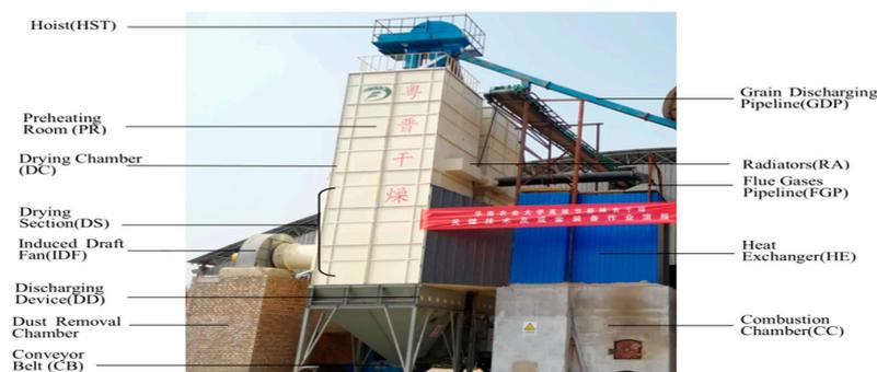
Figure 1. Picture of the industrial drying system.
