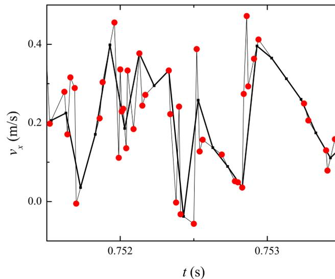
**Figure 2.** Example of raw (circles) and interpolated time series (thick lines). Laser Doppler velocimetry measured the flow velocity at random times. Therefore, we re-sampled the data using Equation (1) at 10,000 Hz .
