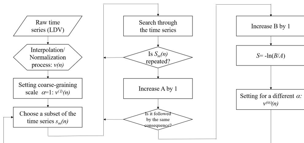
Figure 3. A flowchart to calculate the sample entropy.
