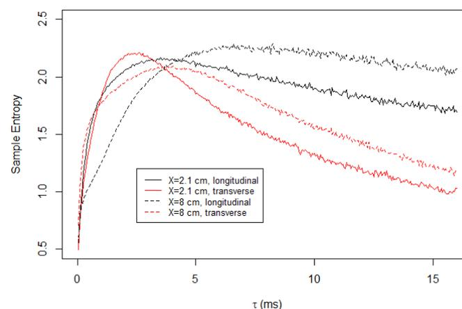
**Figure 4.** Sample entropy calculated for turbulent flow in Soap Film 1. At shorter time scales, the transverse component is more unpredictable. However, at a longer time scale, the opposite is true. We note that the sample entropy naturally decreases with  $\tau$  because the coarse-grained time series are not normalized. The time series is normalized only once for  $\alpha = 1$ .
