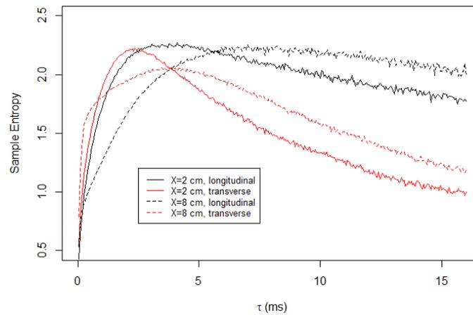
Figure 5. Sample entropy calculated for turbulent flow in Soap Film 2.
