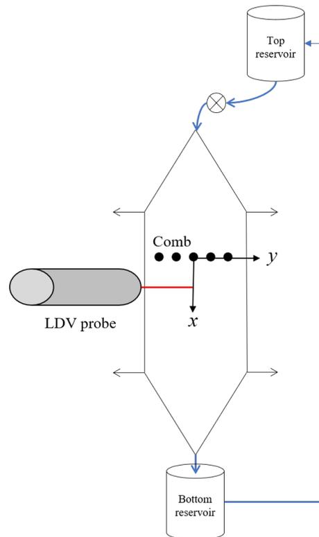
**Figure 1.** Experimental setup. Using a comb, we created a turbulent flow on a flowing soap film channel. The velocity field was measured at several locations downstream of the comb using laser Doppler velocimetry.
