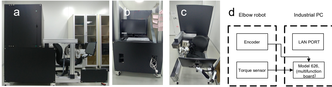
Figure S2. Robot system: (a, b, c) Packaged robot system pictures. (a) is a side view of the packaged robot system, (b) is a rear view of the packaged robot system, where is the operator's workspace, and (c) is a front view of the packaged robot system, where is the subject's workspace; (d) Robot and industrial PC connections. Robot system provides position data from encoder and measured torque data from torque sensor. Position data is digital signals of two channel and torque data is an analog signal.
