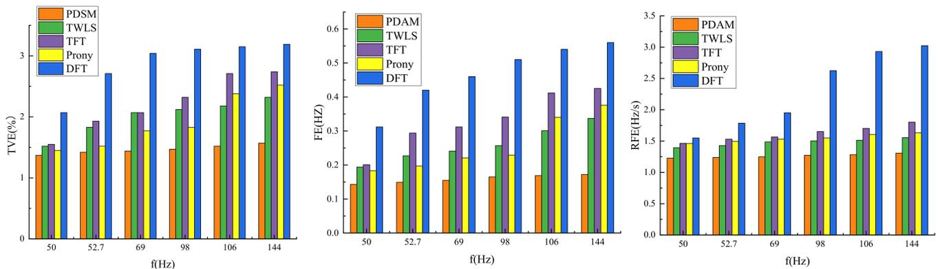
**Figure 3.** The maximum TVE, FE, and RFE of different methods under the frequency ramp condition.
