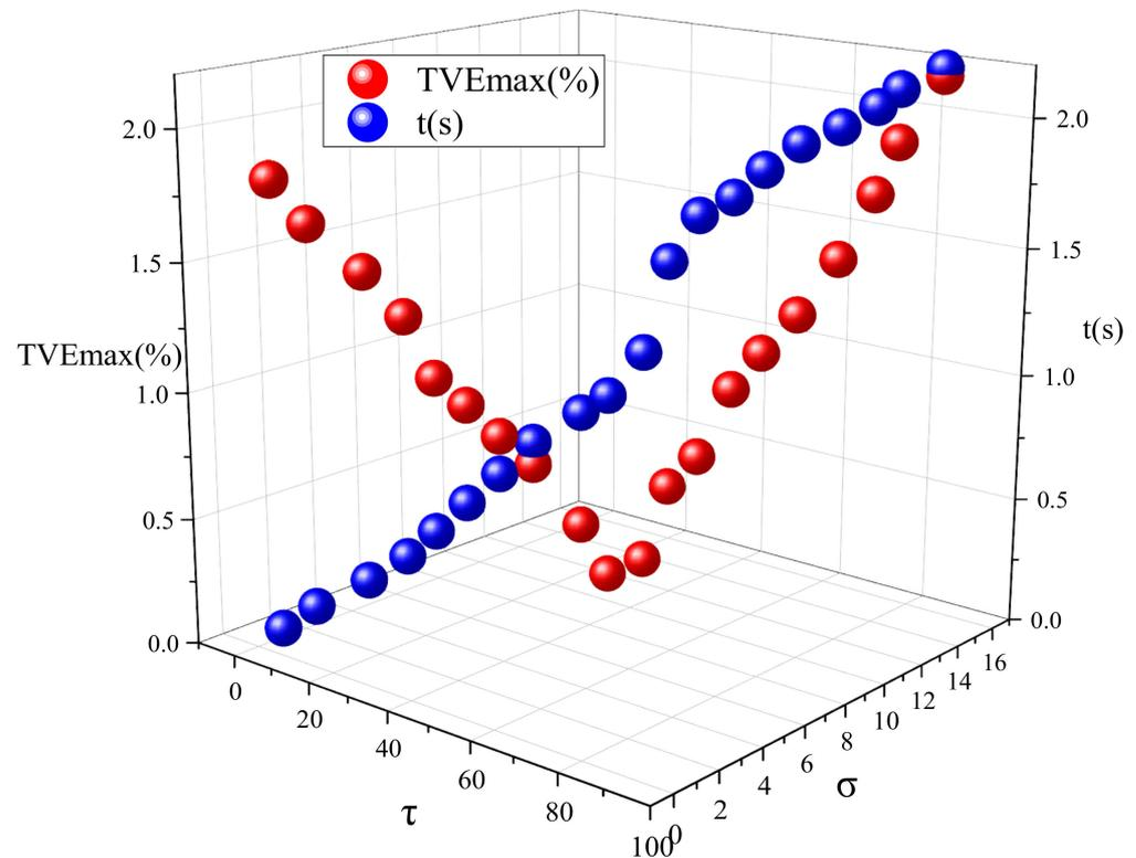
**Figure 1.** Total vector error and operation time with different iteration parameters.
