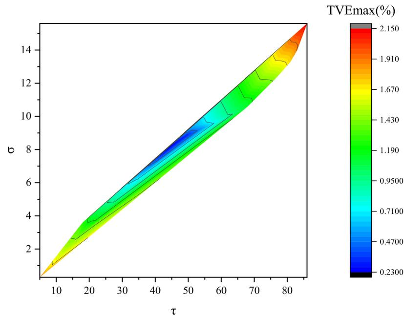
Figure 2. Total vector error with different iteration parameters.
