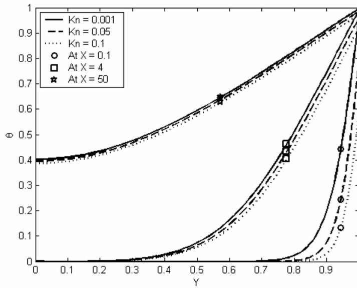
**Figure 5** Spatial temperature profiles at different axial locations and at different Knudsen numbers:  $Re = 200$ ,  $Pr = 0.7$ ,  $Ec = 0.01$ ,  $\sigma_v = 0.7$ ,  $\sigma_T = 0.7$ ,  $\gamma = 1.4$ .
