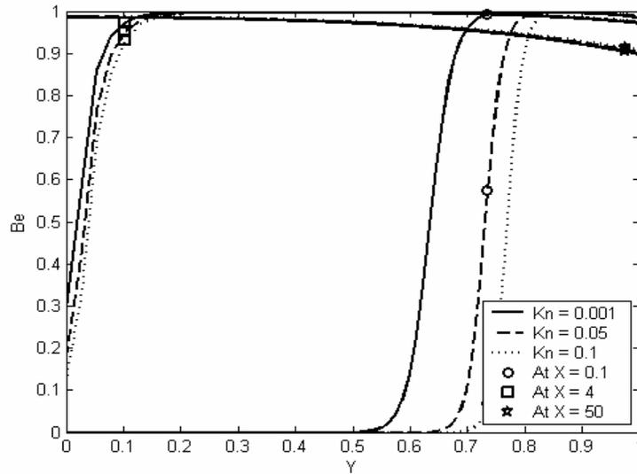
**Figure 7** Spatial distribution of the local Bejan number profiles at different axial locations and at different Knudsen numbers:  $Re = 200$ ,  $Pr = 0.7$ ,  $Ec = 0.01$ ,  $\sigma_v = 0.7$ ,  $\sigma_T = 0.7$ ,  $\gamma = 1.4$ .
