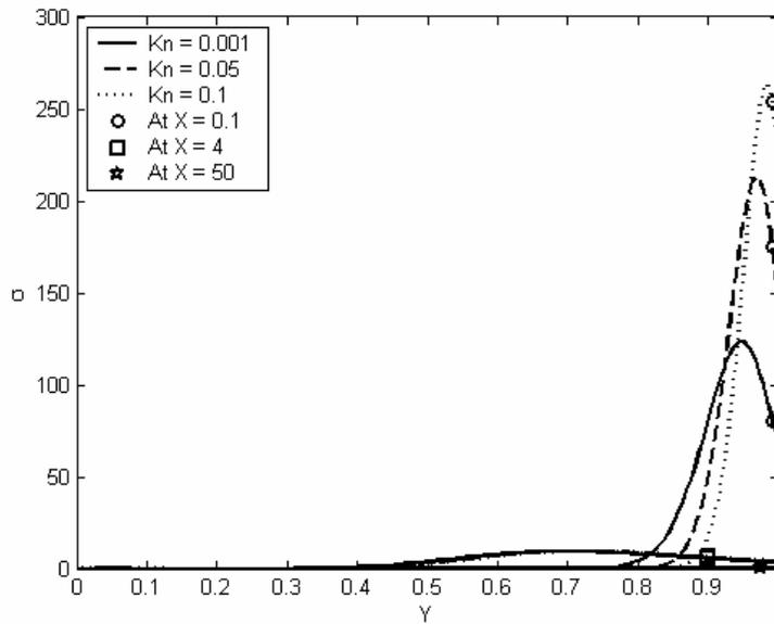
**Figure 6** Spatial distribution of the local entropy generation profiles at different axial locations and at different Knudsen numbers:  $Re = 200$ ,  $Pr = 0.7$ ,  $Ec = 0.01$ ,  $\sigma_v = 0.7$ ,  $\sigma_T = 0.7$ ,  $\gamma = 1.4$ .
