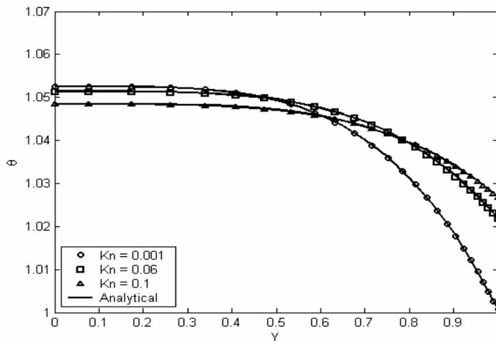
**Figure 3** Comparison of the numerical and analytical solutions of the spatial temperature profiles at different Knudsen number:  $Ec = 0.01$ ,  $Pr = 0.7$ ,  $Re = 50$ ,  $\sigma_v = 0.7$ ,  $\sigma_T = 0.7$ ,  $\gamma = 1.4$ .
