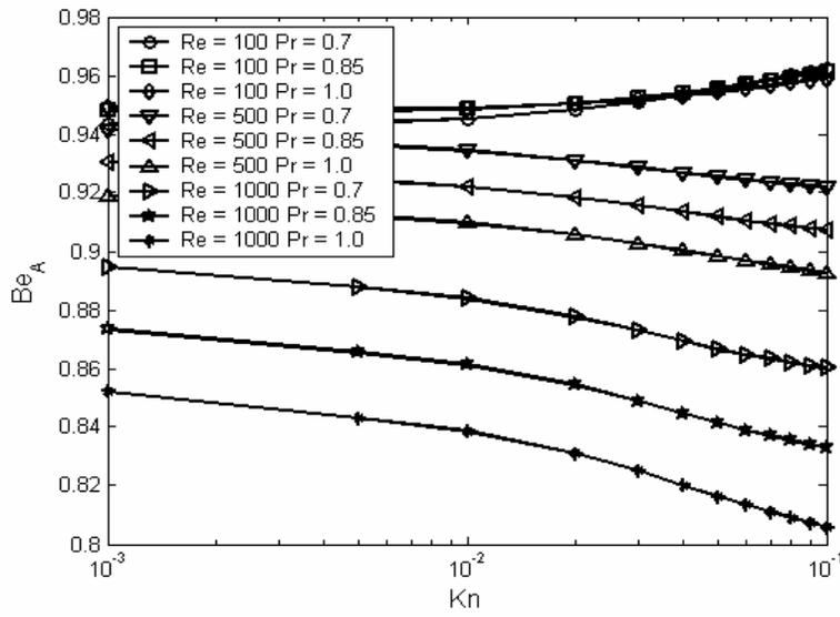
**Figure 10** The average Bejan number as function of Knudsen number and for different values of Reynolds and Prandtl numbers:  $Ec = 0.01$ ,  $NTD = 4$ ,  $\sigma_v = 0.7$ ,  $\sigma_T = 0.7$ ,  $\gamma = 1.4$ .
