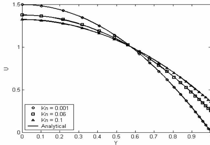
**Figure 2** Comparison of the numerical and analytical solutions of the spatial velocity profiles at different Knudsen numbers:  $Ec = 0.1$ ,  $Pr = 0.7$ ,  $Re = 50$ ,  $\sigma_v = 0.7$ ,  $\sigma_T = 0.7$ ,  $\gamma = 1.4$ .
