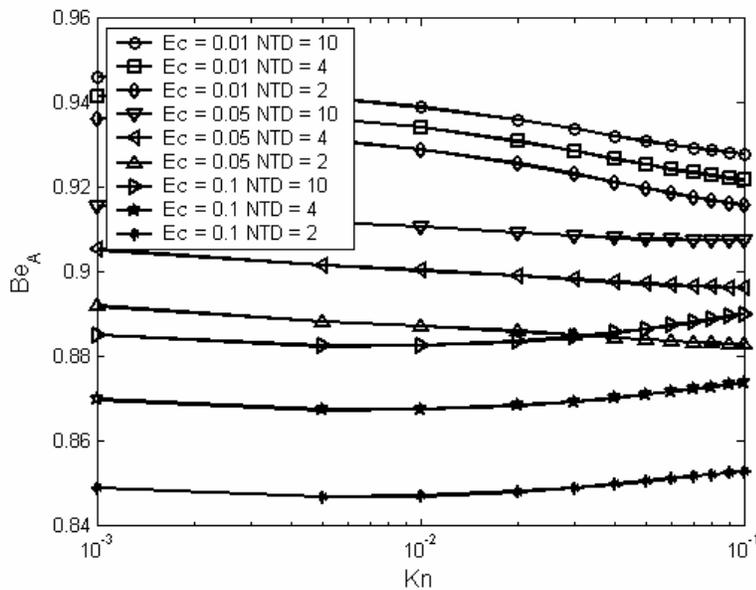
**Figure 11** The average Bejan number as function of Knudsen number and for different values of Eckert number and NDT:  $Re = 500$ ,  $Pr = 0.7$ ,  $\sigma_v = 0.7$ ,  $\sigma_T = 0.7$ ,  $\gamma = 1.4$ .
