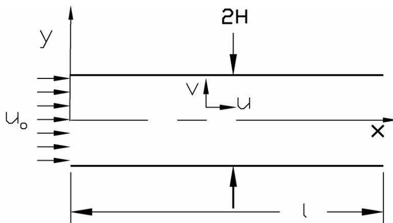
**Figure 1** Schematic drawing of the problem geometry.
