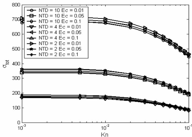
**Figure 9** The total entropy generation as function of Knudsen number and for different values of Eckert number and NDT:  $Re = 500$ ,  $Pr = 0.7$ ,  $\sigma_v = 0.7$ ,  $\sigma_T = 0.7$ ,  $\gamma = 1.4$ .
