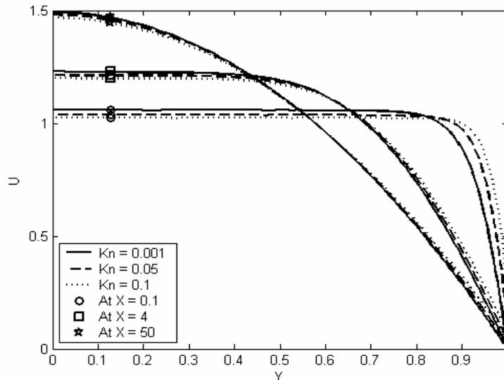
**Figure 4** Spatial velocity profiles at different axial locations and at different Knudsen numbers:  $Re = 200$ ,  $Pr = 0.7$ ,  $Ec = 0.01$ ,  $\sigma_v = 0.7$ ,  $\sigma_T = 0.7$ ,  $\gamma = 1.4$ .
