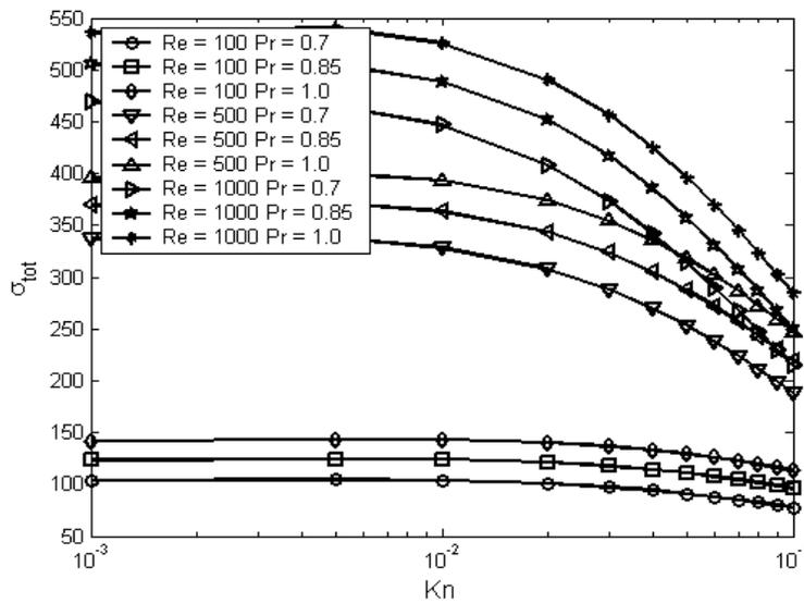
**Figure 8** The total entropy generation as function of Knudsen number and for different values of Reynolds and Prandtl numbers:  $Ec = 0.01$ ,  $NDT = 4$ ,  $\sigma_v = 0.7$ ,  $\sigma_T = 0.7$ ,  $\gamma = 1.4$ .
