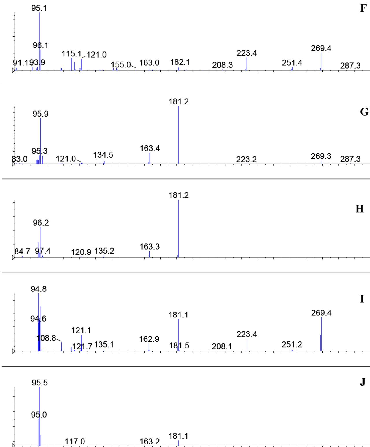
The ionization method used by Merbel *et al.* [14] was APCI, which is more energetic and causes in-source fragmentation, therefore neither pilocarpic nor isopilocarpic acid could be quantified as parent ions ( $m/z$  227), but only as their fragments ( $m/z$  209). The use of a much softer ionization (ESI) permitted the observation of all the compounds based on the mass of the protonated  $[M + H]^+$  molecules, not of fragment ions, which is essential for bio-prospection of new compounds.
